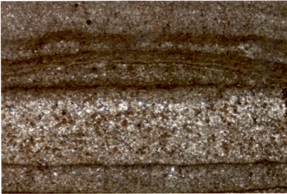
Plate 3. Photomicrograph (X 25) of an algal biolithite (boundstone) representative of microfacies II.
