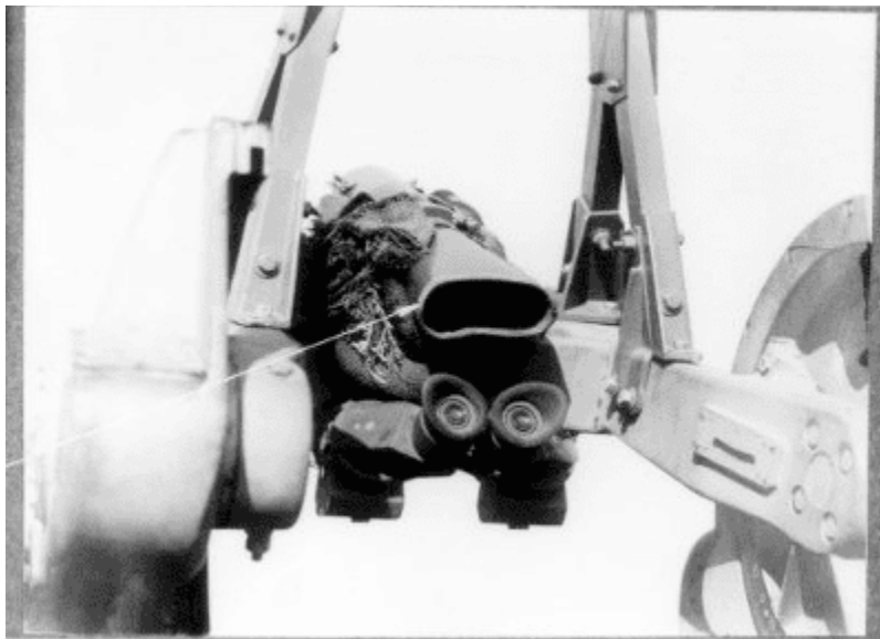
Figure 47. Mark 4 Model 3 fire-control radar transmitter captured on Saipan, scope, July 1944 (Land Radar of the Japanese Navy 2018).
