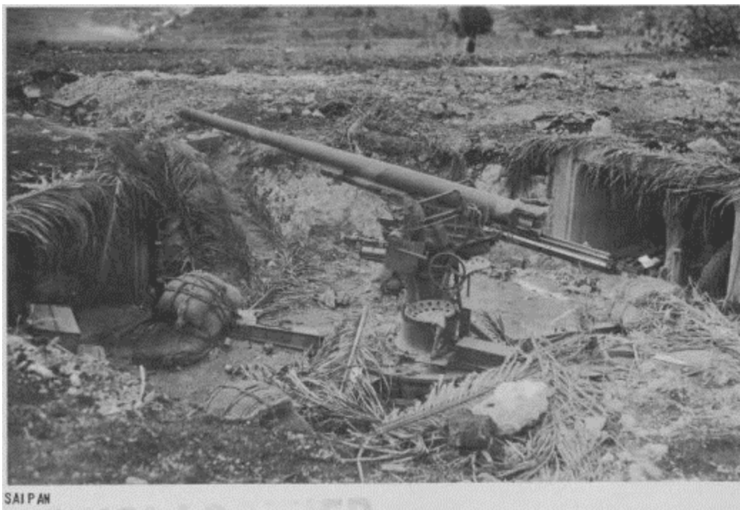
Figure 20. Type 88 75 mm. AA gun captured on Saipan (Office of the Chief of Naval Operations 1945b).
