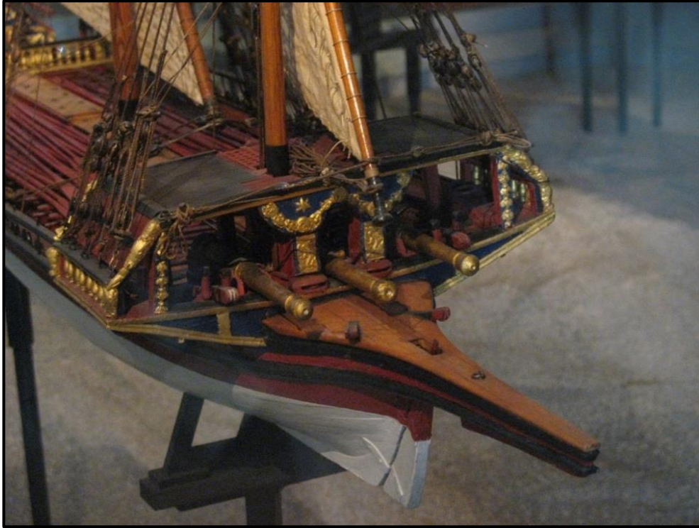
FIGURE 10: Rambade on stern of model of early 18th century Swedish galley by Axel Lewenhaupt circa 1715 (NMMS 2025).
