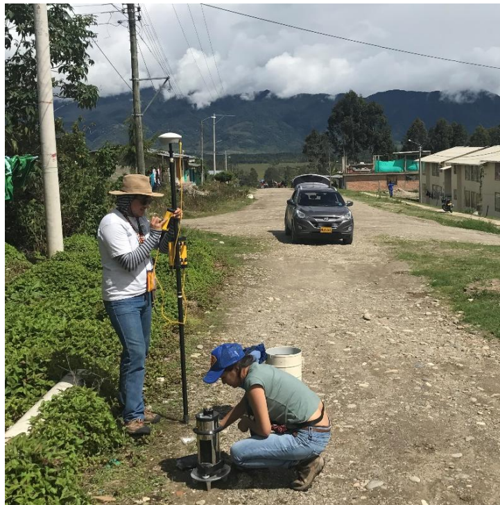
Figure 12 Worden gravimeter, next to differential GPS at a station in the Sibundoy Valley, Colombia. Acknowledgement for Nicolas Perez, Andrea Ordonez for help with the field measurements and to Camilo Jaramillo for overall project support.
