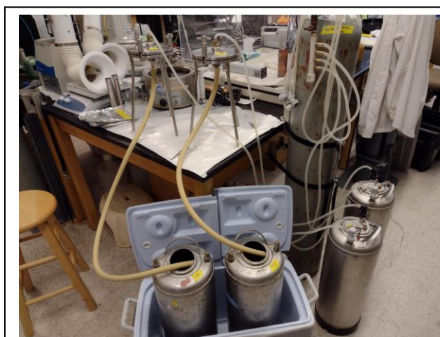
Fig. 2.4: The filtration rig used to filter samples, the two tanks with lids on the left are the water samples, and the two tanks in the cooler are used to collect wastewater, the two tripods are filter heads and will contain the retentate.
