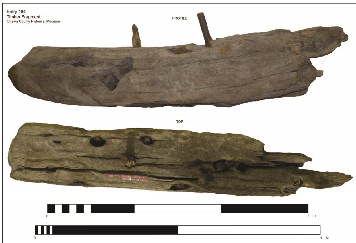
FIGURE 6.12. Entry 194 teak timber fragment with iron nails and trunnels recorded by the author at the Ottawa County Historical Museum on 31 August 2011.
