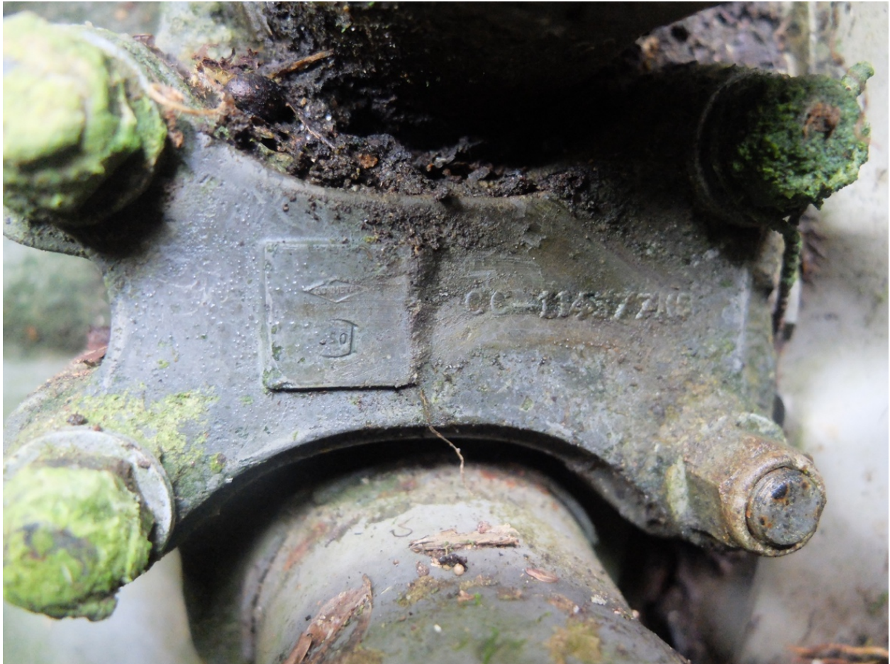
Figure 34: Jungle site part 114377NS – COVER: Engine mounting bracket substituting (United States Air Force 1952:73) (Photograph by Author)
