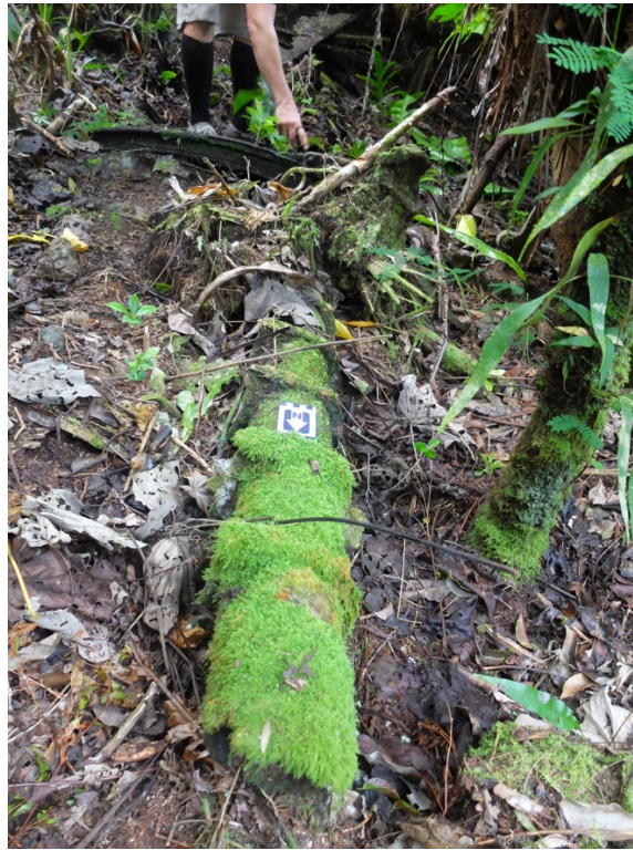
Figure 40: Tube assembly track support Part 8-2053 with wing flap tracks Part 14-2224 (United States Air Force 1950:15), jungle site (Photograph by Peter Harvey)
