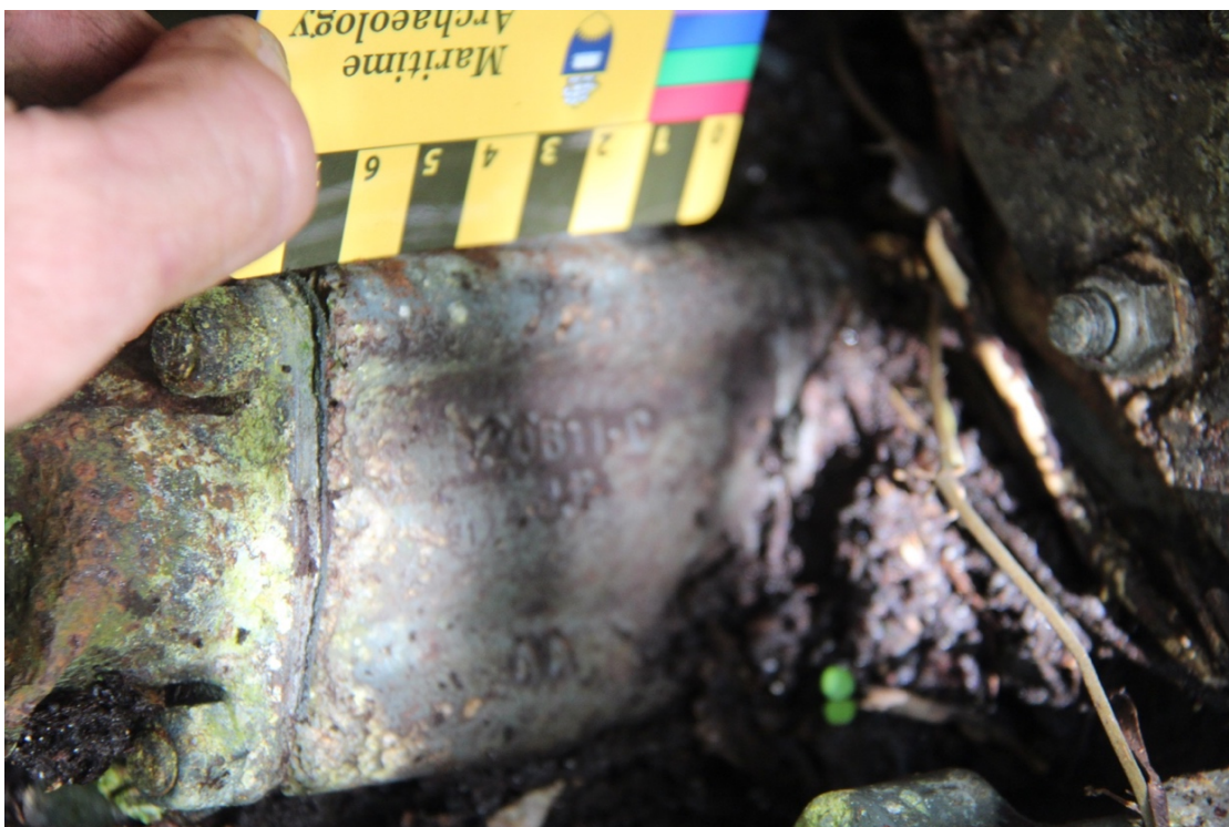
Figure 36: Jungle site part 120611-C ADAPTER: Rear oil pump external oil inlet tube (United States Air Force 1952:125) (Photograph by Author)
