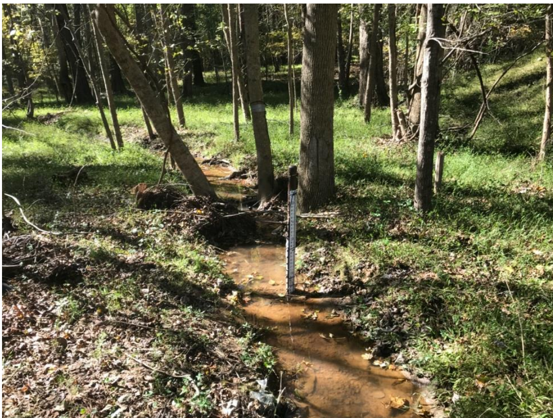
Figure 5. Staff gauge with a water-depth logger installed in it.
