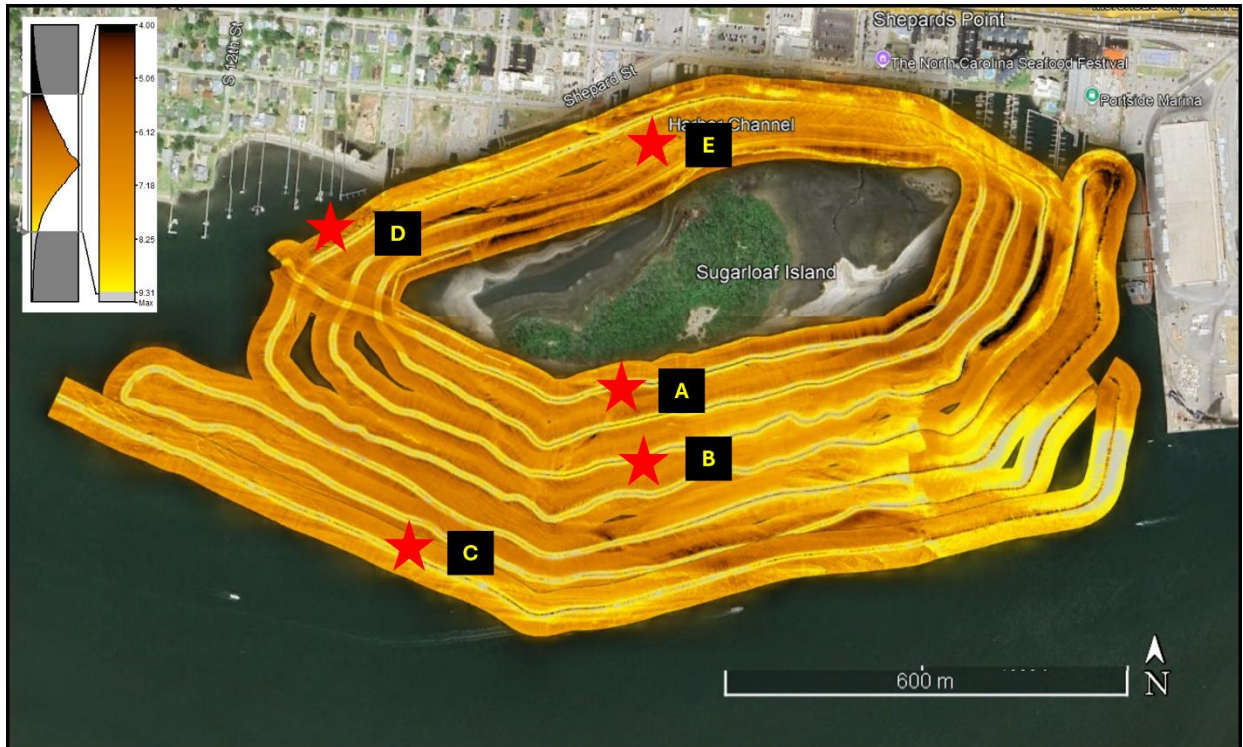
Figure 14. Side-scan sonar mosaic. Darker shades represent finer sediments; lighter shades represent coarser sediment. Made using SonarWiz ver. 7 and Google Earth. Close-up images of points A, B, C, D, E, and F can be found in figure 16.
