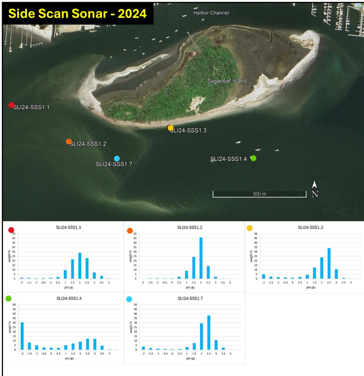
Figure 17. Map of the sediment sample sites with respective histograms illustrating the distribution of sediment sizes (in phi) by weight percent of Side Scan Sonar sediment samples. Each colored dot relates to a corresponding histogram with the same-colored dot. Enlarged histograms are shown in Appendix A, Figure A4.
