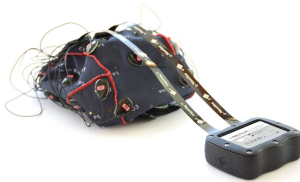
Figure 11: g.Tec Nautilus wireless EEG headset [44].
