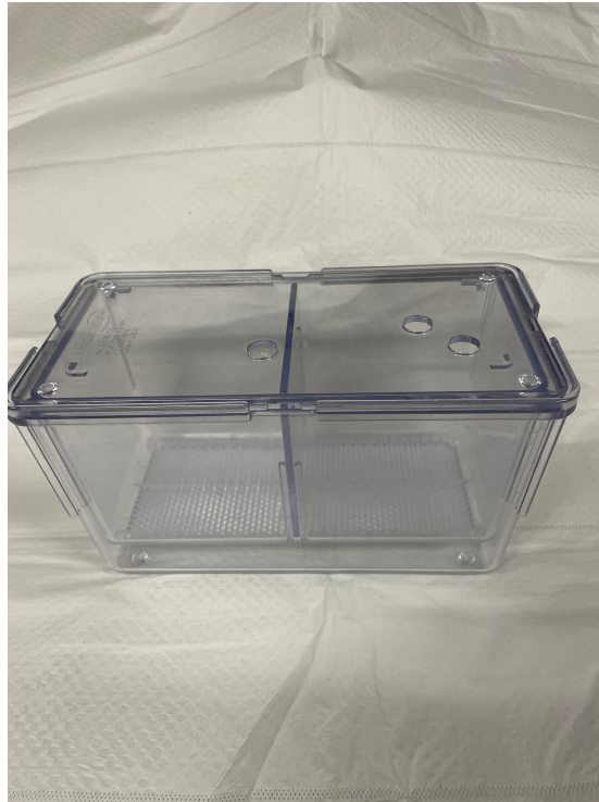
Figure 8 – Static Zebrafish Breeding Tank - Embryos generated fall through the perforated insert and are collected at the bottom. The insert is removable so that the adult fish can be moved to a fresh tank and the embryos harvested.
