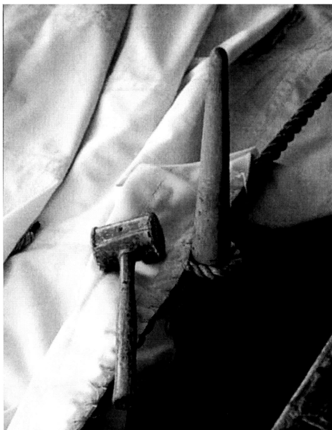
Figure 42. 1997 USS Constitution sail cringle stretched on a setting fid. (Photograph by N. S. Wilson.)
