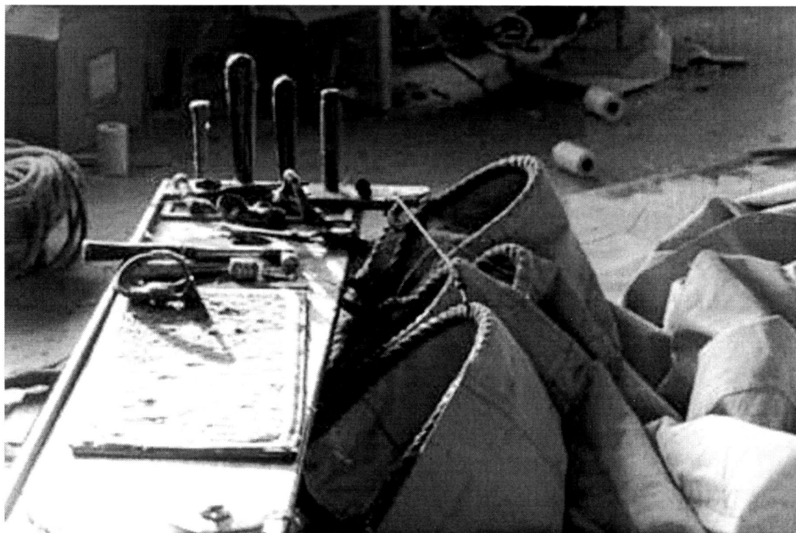
Figure 34. Sailmaker's bench with bench hook in the sail's boltrope. (Photograph by N. S. Wilson of the Mayflower II 's hand-stitched cotton sails.)
