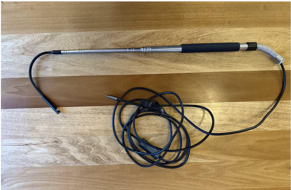
Figure 13. The bore cam, a Teslong Telescopic Pole Inspection Camera, was utilized by James Fowler to inspect the interior of the cannon barrels. (Photo by James Fowler.)
