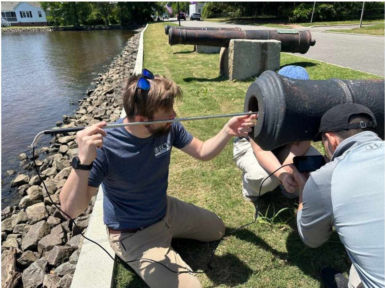
Figure 15: James Fowler utilizes the bore cam on a cannon in Edenton, NC. Addison Costa (foreground) views the live feed through a phone app. (Photo by Abigail Fowler.)
