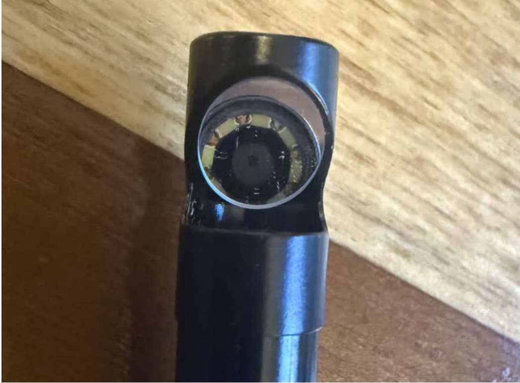
Figure 14. The mirror attachment that allowed the Bore Cam to view ninety-degrees to the axis. (Photo by James Fowler.)
