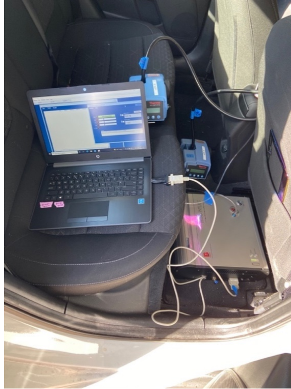
Figure 2(c) Back seat of the vehicle displaying the aerosol monitoring equipment set-up
