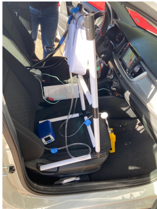
Figure 2(a) Vehicle Schematic displaying the aerosol monitoring equipment set-up
