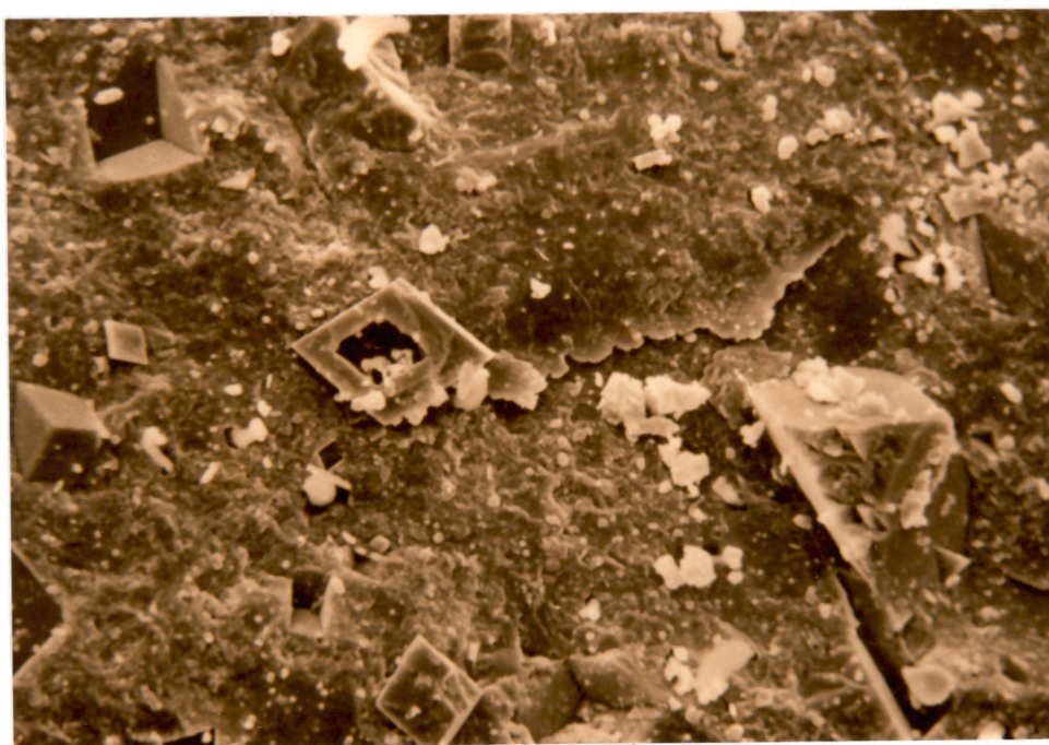
Plate 22. Hollow dolomite in chert nodule. Core OB-35, 8.00m. (SEM photomicrograph, 1500x)
