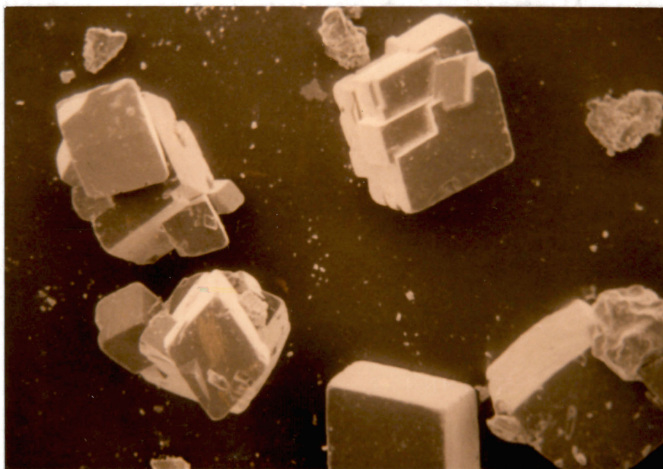
Plate 18. Euhedral dolomite rhombs in the BBF sequence. Notice the plane, even surfaces of the rhombs. Core OB-1, 4.50-4.75m. (SEM photomicrograph, 1000x)
