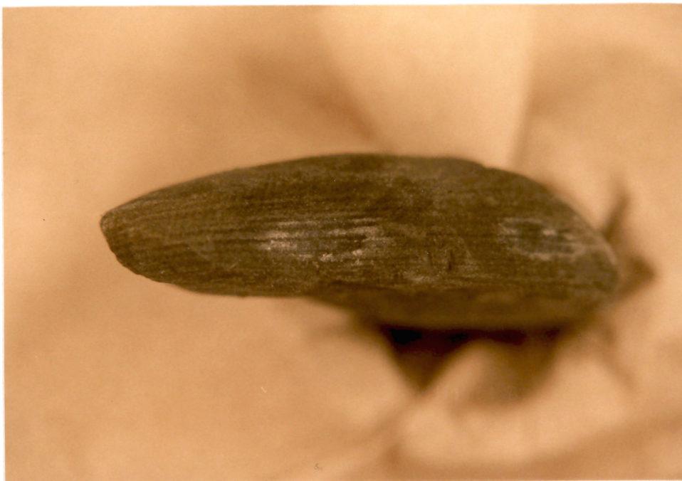
Plate 28. Chert nodule showing bedding preserved by silicification. Core OB-123, 5.00-5.25m. Nodule is 7cm long.
