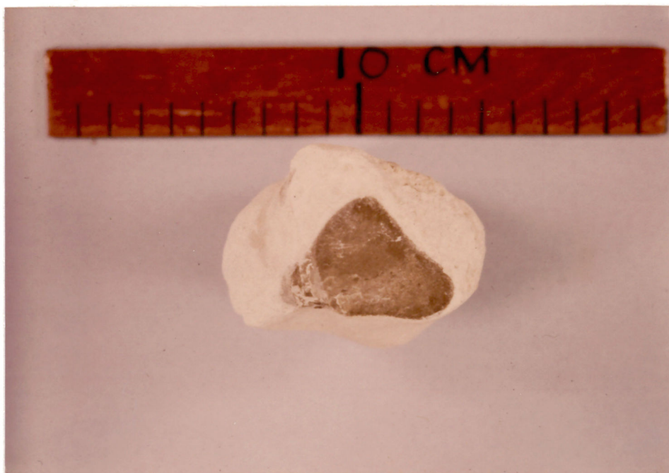
Plate 23. Chert nodule from seismic unit AF-1. The gray central area of the nodule is the silicified part; the white outer rim is calcite cemented, dominantly unreplaced carbonate sediment. Core OB-35, 8.00m.
