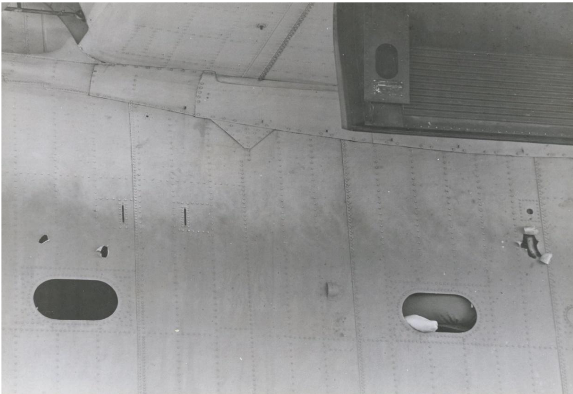
FIGURE 2.18: Damage to aircraft 16-P-1 documented while aboard Pokomoke . Note outward bending metal on airframe skin indicating bullet exit holes (Photo courtesy of National Archives photo #80-G-234456).
