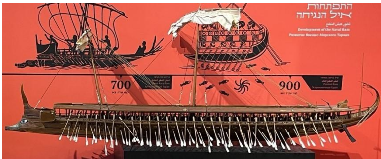
Figure 6.1: Model of a trireme at the National Maritime Museum, Haifa, Israel. The model has a symbolic or apotropaic eye (see below), ram at the bow, with a steering oar at the stern. This representation was modeled after the Atlit ram and its reconstructed ship (photo by M. Elsner in 2023).
