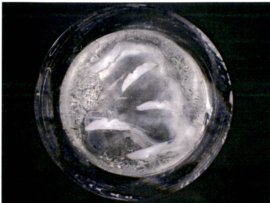
Figure 4. Southern flounder otoliths mounted in 25-mm Plexiglas ring mounts. Sectioned otoliths were mounted in ring mounts to be polished prior to conducting LA-ICP-MS. Usually 5 otoliths were embedded per ring mount.
