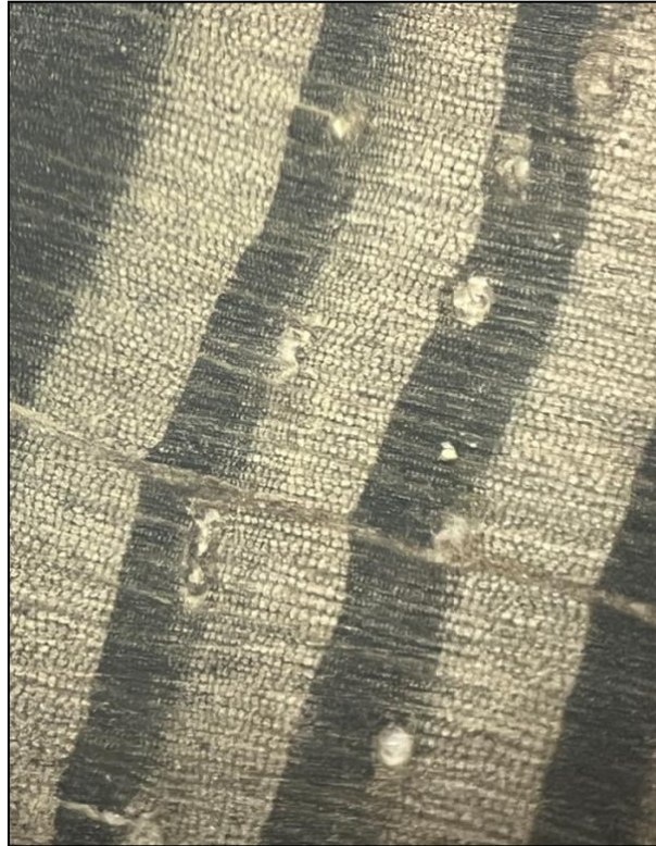
FIGURE 31: Microscopic image of core sample CAS013. The diagnostic features of high resin context and pronounced latewood banding are visible (Photo courtesy from author, 2024).
