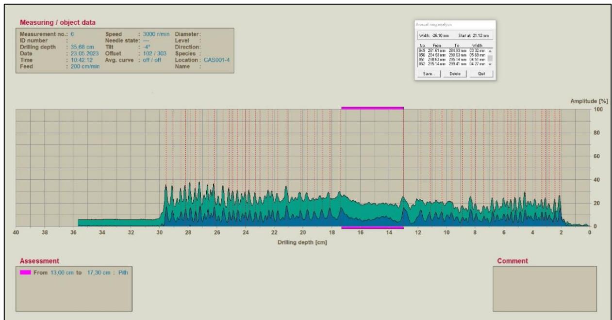
FIGURE 3: RESI Measurement 6 out of the 17 drillings done. This timber is not associated with a core sample (Graph by author, 2023).
