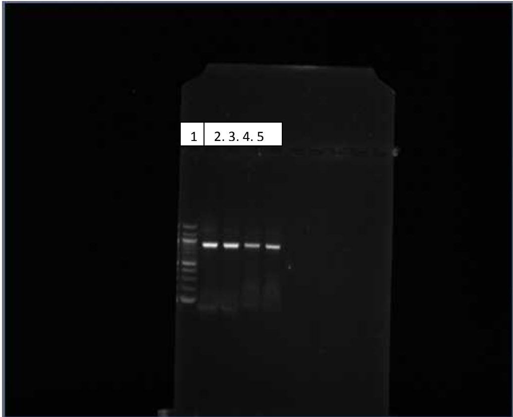
Figure 14: 1% agarose gel showing archaeal 16S rRNA amplicons for WHB. Band size is 937 bases.
