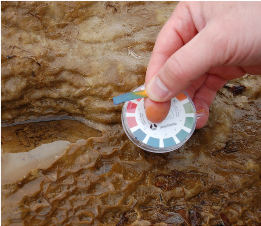
Figure 5: Test strip indicating a pH ~11 for the WHC2 alkaline spring.
