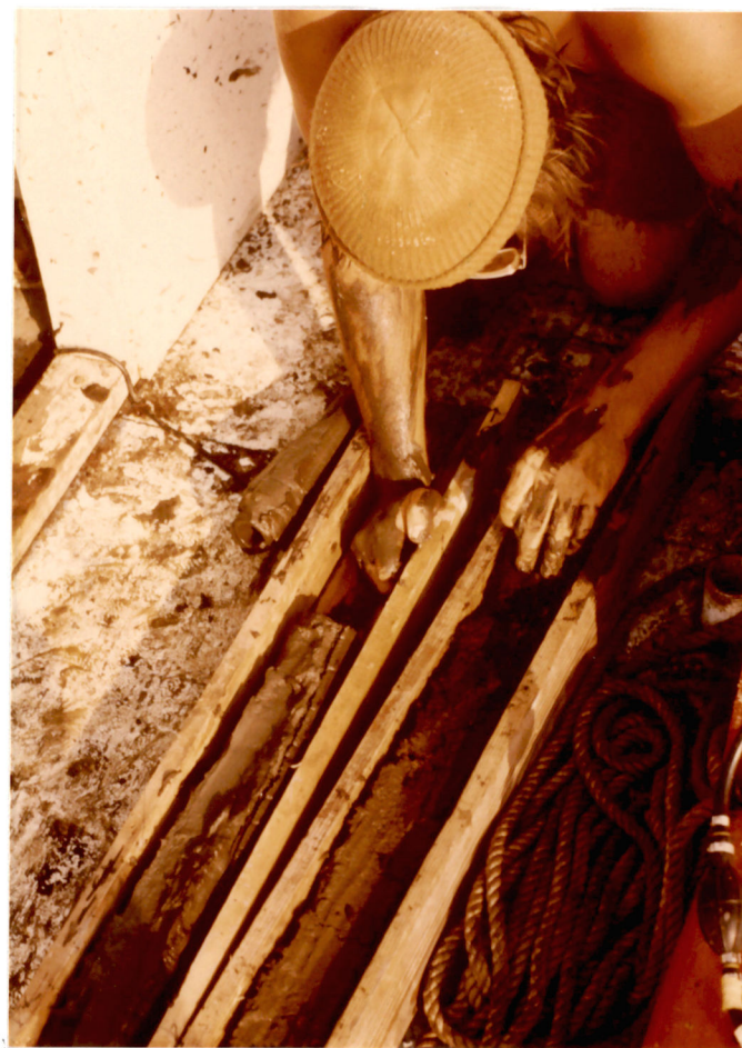
Figure 7. A freshly extruded core. The cores were extruded into plastic lined two meter wooden carriages for transport from the field.
