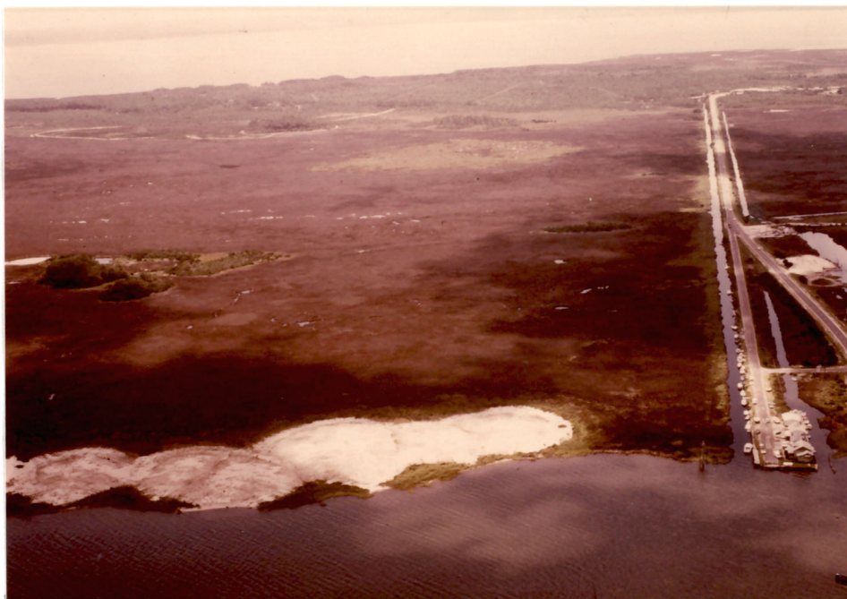
Figure 18. Man-made marsh features. The barren white feature adjacent to the shoreline is a spoil disposal area resulting from the dredging of the shipping channel down Roanoke Sound. The channel which borders the highway was initially dredged to provide fill for the roadbed. It is presently serving the marina complex at the end of the road as boat dockage.
