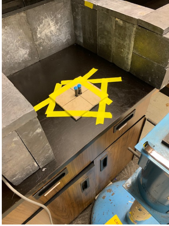
Figure A.1: Gamma Irradiation setup for the calibration of beta source
