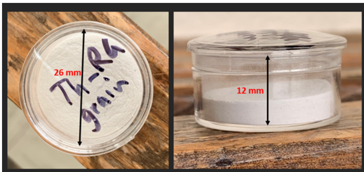
Figure 7.2: The non-infinite matrix sample container with internal diameter of about 26 mm and height of about 12 mm without the cap. Most of the samples in the container had heights of \sim 3 –9 mm.
