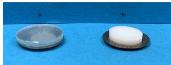
Figure 3. Absorber and sample cup combinations: (a) 12 mm diameter microscope coverslip glass stack on top of the sample cup with a dosimeter and (b) 1.9 mm PTFE disk placed inside the sample cup directly on top of the dosimeter.
