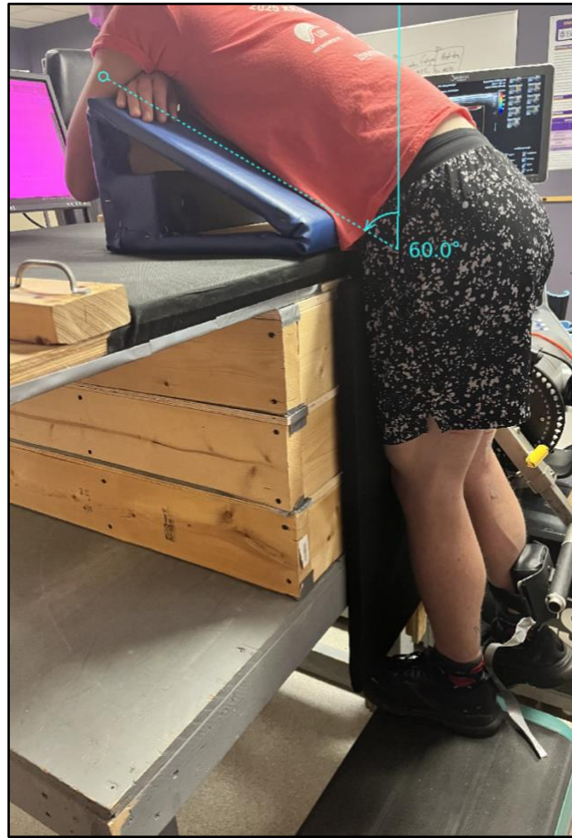
Figure 1. Custom built apparatus, with knee in line with the dynamometer axis of rotation and hip aligned to the apparatus, which consisted of a board and a 30-60-90 triangle. The triangle was rotated to position the hips in 0°, 30°, and 60° of hip flexion.
