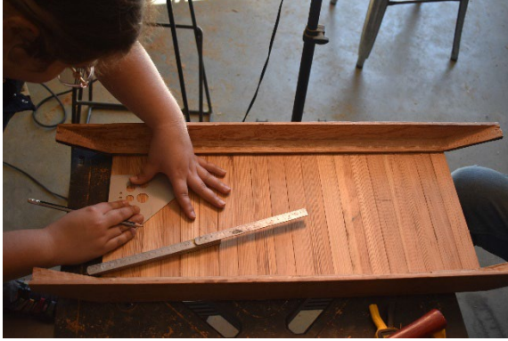
PHOTO 25. Saldivar measuring a marking where the stringer pieces should rest (Photo by Michaela Hoots).
