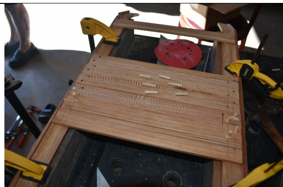
PHOTO 18. Scale model upside down showing treenails being driven into planking and chine-girder (Photo by Alyssa Saldivar).
