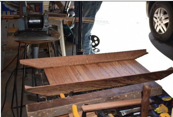
PHOTO 21. Chine-girder resting on its bottom, exterior planking for ramps not added (Photo by Michaela Hoots).
