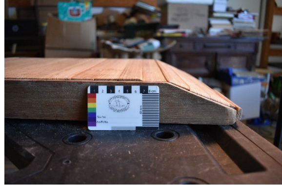
PHOTO 50. Photo of vessel resting upside down with photo scale to show the angle of the ramp (Photo by Michaela Hoots).
