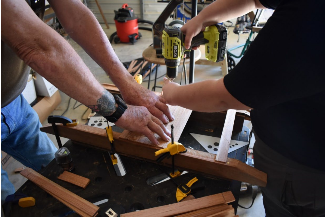
FIGURE 36. Photo showing the hull planking being placed on to the chine-girders (Photo by Michaela Hoots).
