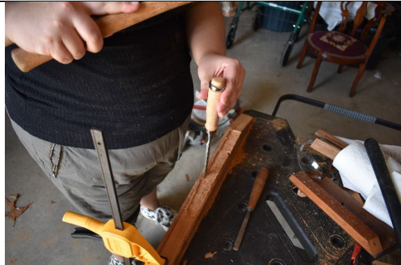
PHOTO 4. Saldivar using a hammer and chisel to cut the rabbet of the chine-girder (Photo by Mark Newell).
