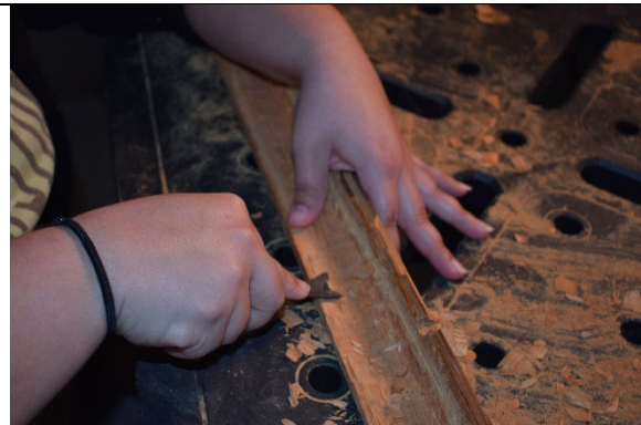
PHOTO 10. Saldivar using a carving tool to carve out the interior shelf of the chine-girder (Photo by Mark Newell).
