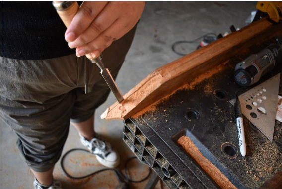
PHOTO 5. Saldivar using a hammer and chisel to cut a hard-right angle into the rabbet of the chine-girder (Photo by Mark Newell).
