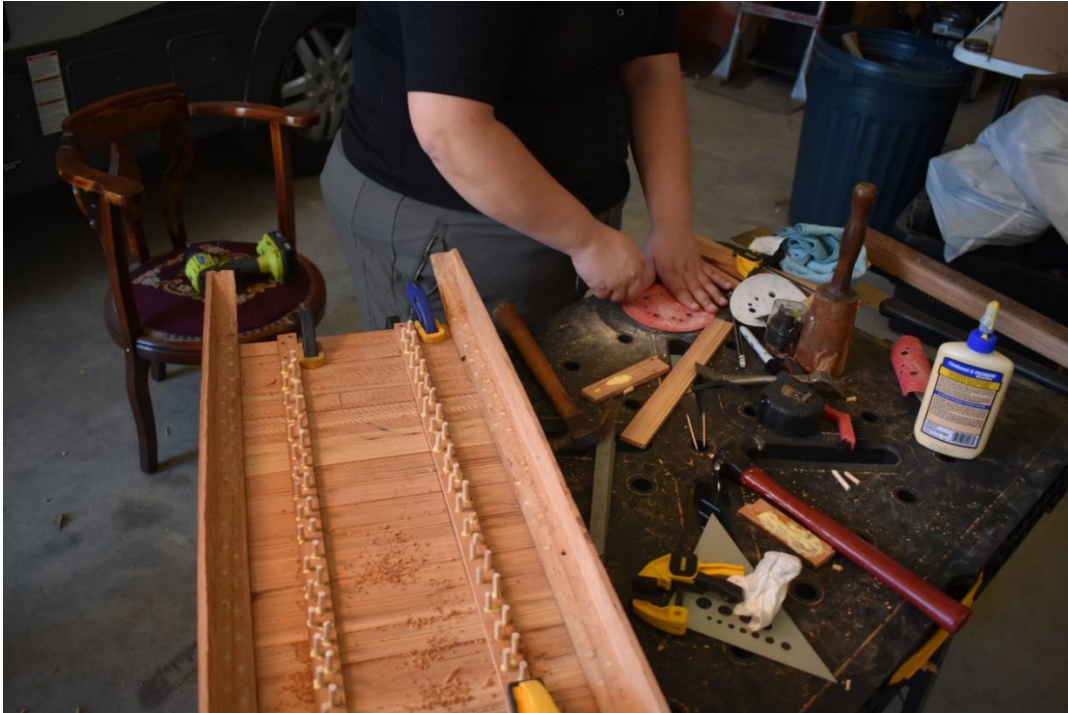
FIGURE 39. Photo showing the stringers placed on top of the hull planking, with treenails through the stringers and hull planking (Image by Mark Newell).
