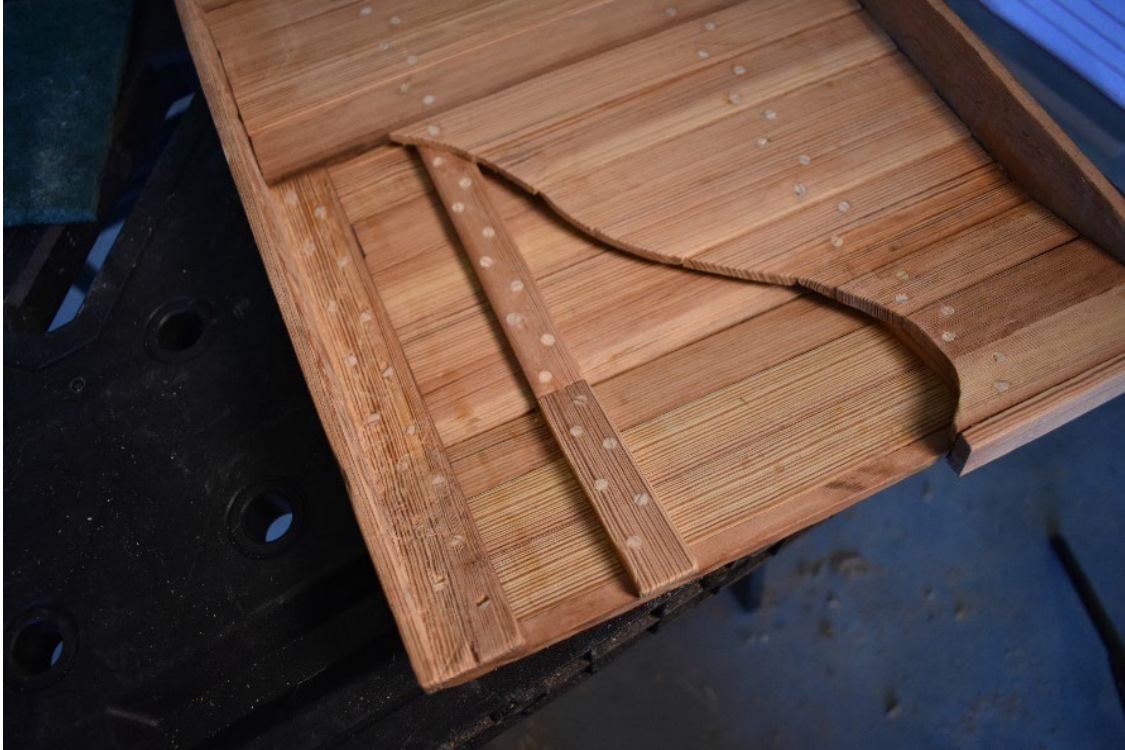
FIGURE 42. Photo of the near-completed scale model of the Oconee River flatboat, showing the cut-out chosen so the inside construction of the vessel could be seen (Image by Alyssa Saldivar).
