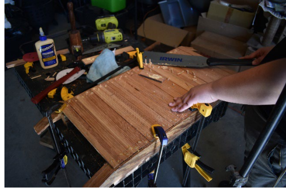
PHOTO 20. Saldivar cutting away excess treenail length (Photo by Michaela Hoots).
