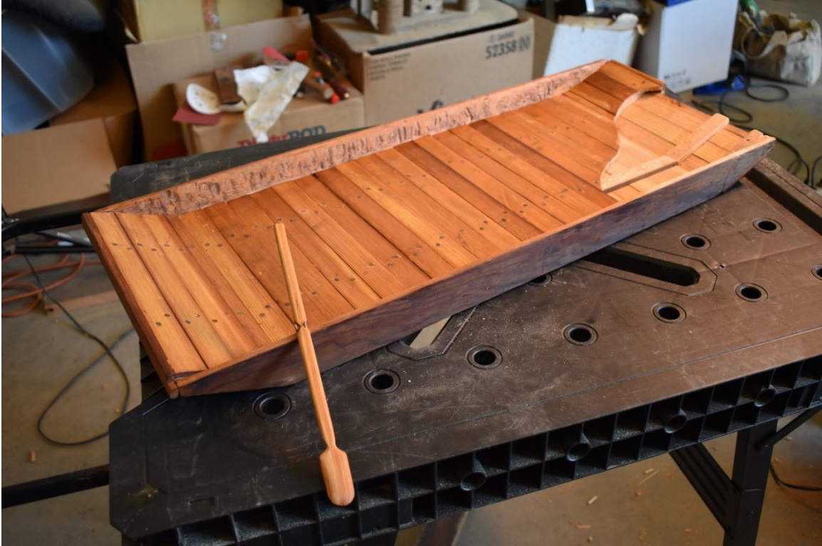
FIGURE 43. Photo showing the one thole pin pairing, and the finished model (Photo by Alyssa Saldivar).
