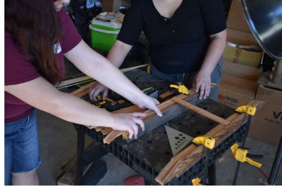
PHOTO 14. Saldivar and Hoots setting the hull planking into the rabbets of each chine-girder (Photo by Mark Newell).
