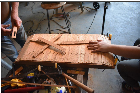
PHOTO 35. Saldivar and Newell fitting exterior ramp planking to the vessel (Photo by Michaela Hoots).
