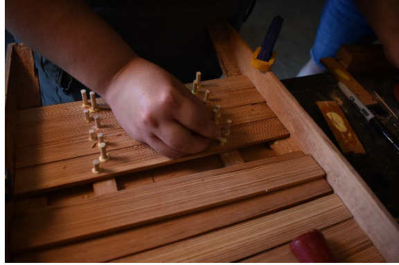
PHOTO 32. Saldivar inserting treenails into interior planking and stringers (Photo by Michaela Hoots).
