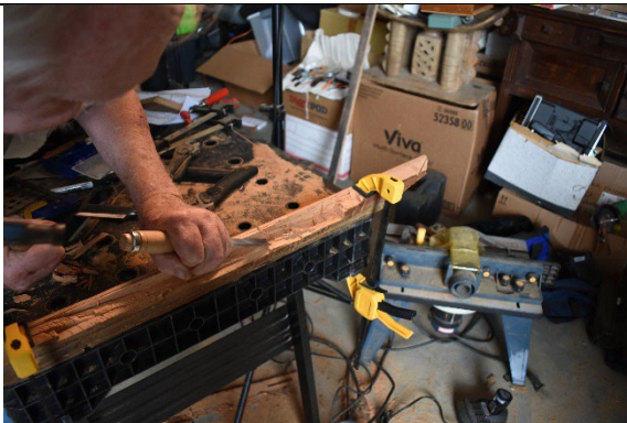
PHOTO 9. Newell using a hammer and chisel to carve out the interior shelf of the chine-girder (Photo by Alyssa Saldivar).
