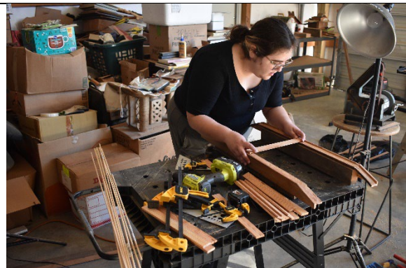
PHOTO 12. Saldivar setting the hull planking into the rabbets of each chine-girder (Photo by Michaela Hoots).
