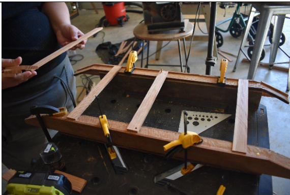
PHOTO 15. Saldivar setting the hull planking into the rabbets of each chine-girder (Photo by Michaela Hoots).
