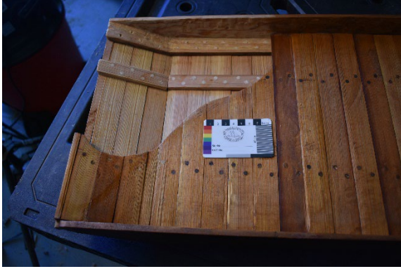
PHOTO 55. Photo of the completed vessel, highlighting the cut out where the interior construction can be seen (Photo by Alyssa Saldivar).
