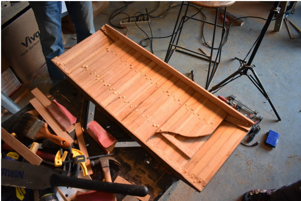
FIGURE 41. Photo showing the hull planking for the ramp attached (Image by Alyssa Saldivar).
