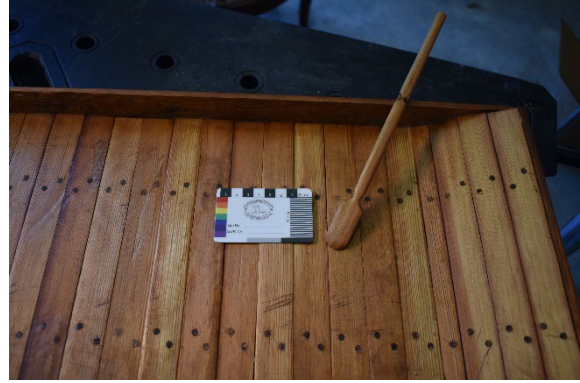
PHOTO 56. Photo of the completed vessel, highlighting the thole pins and the sweepstick (Photo by Alyssa Saldivar).
