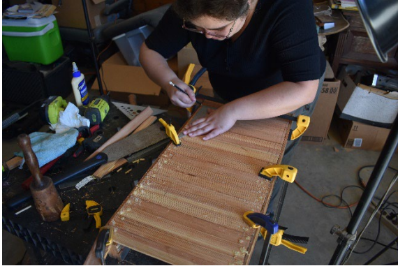
PHOTO 19. Saldivar marking the location of where holes will be drilled for treenails (Photo by Michaela Hoots).
