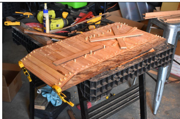
PHOTO 36. Photo of finished exterior planking (Photo by Michaela Hoots).
