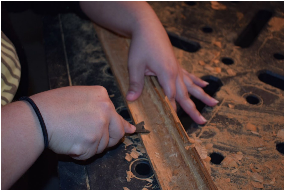
FIGURE 35. Photo showing the author hand carving the hard-right angle of the chine-girder (Image by Mark Newell).
