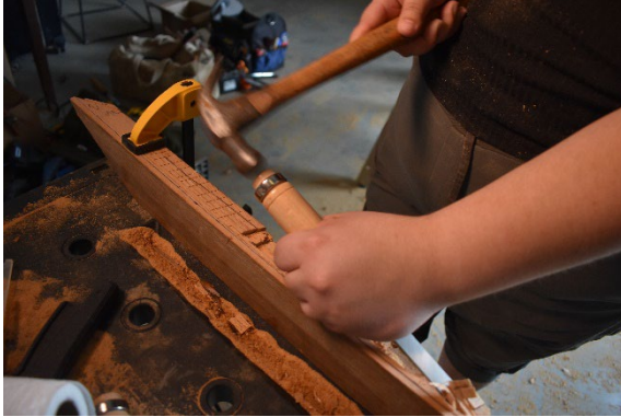
PHOTO 7. Saldivar using a hammer and chisel to carve out the interior shelf of the chine-girder (Photo by Mark Newell).
