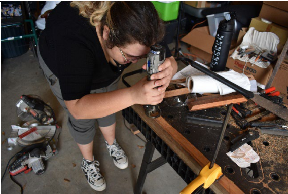
PHOTO 3. Saldivar using a Dremel to cut the rabbet into the bottom of one of the chine-girders (Photo by Mark Newell).
