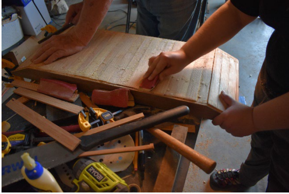
PHOTO 37. Saldivar and Newell sanding down treenails on exterior planking (Photo by Michaela Hoots).
