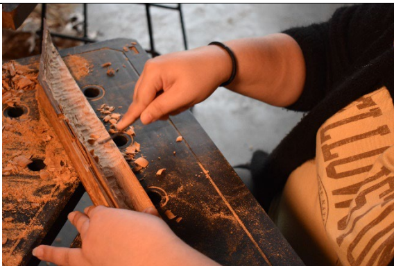
PHOTO 11. Saldivar using a carving tool to carve out the interior shelf of the chine-girder (Photo by Mark Newell).
