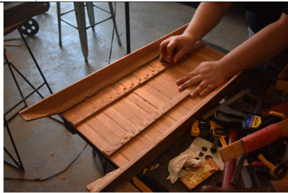
PHOTO 26. Stringer pieces in place and fastened to exterior planking with four treenails for each plank (Photo by Michaela Hoots).
