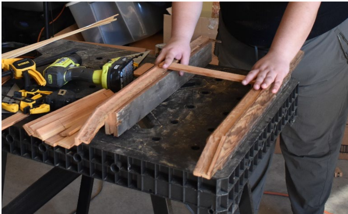
FIGURE 37. Photo showing the chine-girders placed on their gunnels so the hull planking could be laid in (Photo by Michaela Hoots).
