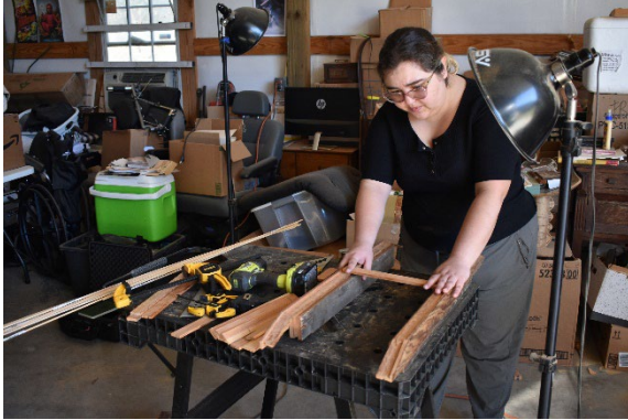
PHOTO 13. Saldivar setting the hull planking into the rabbets of each chine-girder (Photo by Michaela Hoots).
