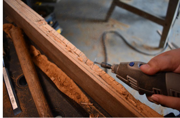
PHOTO 8. Saldivar using a Dremel to carve out the interior shelf of the chine-girder (Photo by Mark Newell).
