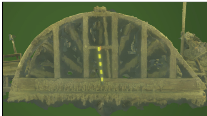
FIGURE 92. Finnish paddle steamer Diana 's paddle box framing. Note the five king posts and flared after section (courtesy of Topi Sellman, Maritime Archaeological Society of Finland).
