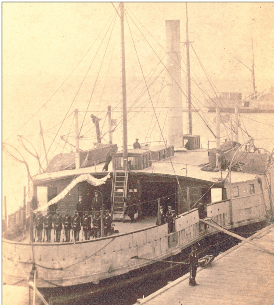
FIGURE 87. Photograph circa 1863 of unidentified union gunboat. Note the low height of the main cabin and the pilot houses dropped into the main cabin (courtesy of the Liljenquist Family Collection of Civil War Photographs, the Library of Congress Archives, Washington D.C.; reference # LOT 14043-2, no. 74).
