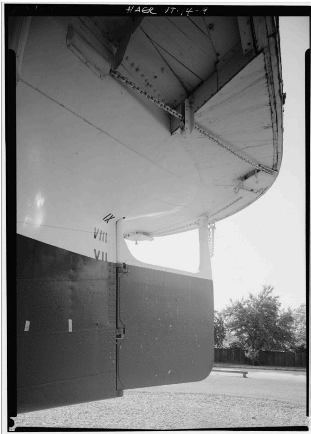
FIGURE 83. Port side view of rudder and steering chain system of steamer Ticonderoga (courtesy of the Historic American Engineering Record, Library of Congress Prints and Photographs Division, reference # HAER VT,4-SHEL,1-9).
