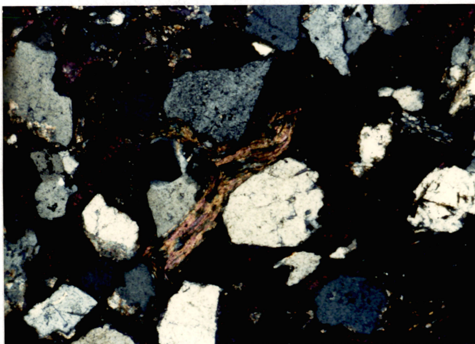
Plate 11. Photomicrograph of a "squeezed" micaceous metamorphic rock fragment around corroded and partially replaced (by calcite) quartz grains.
