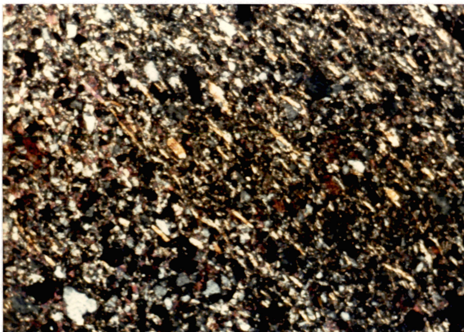
Plate 12. Photomicrograph of an argillaceous siltstone which has undergone compaction as evidenced by the strong alignment of the elongate muscovite grains.
