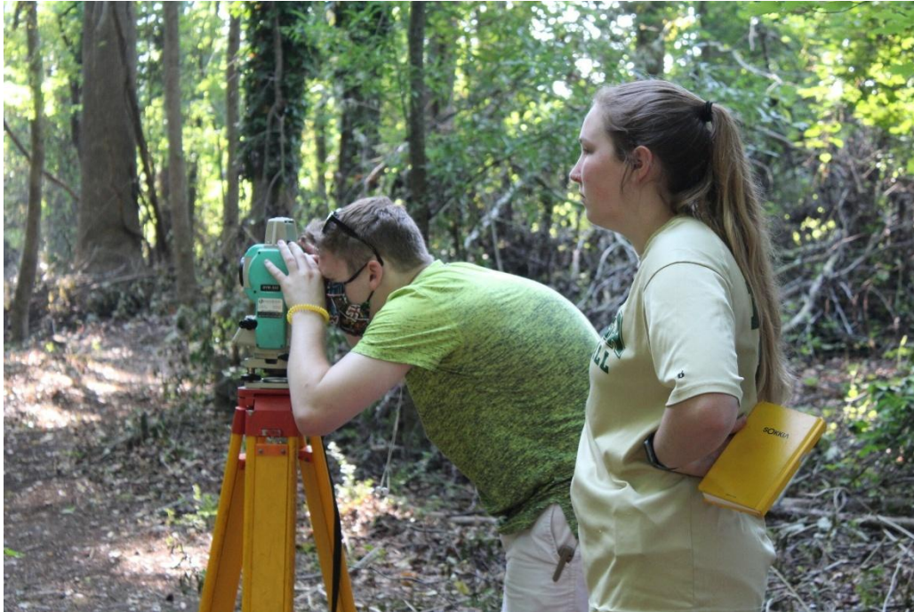
Figure 3.6: ECU students record markers at the 4AC using a total station
