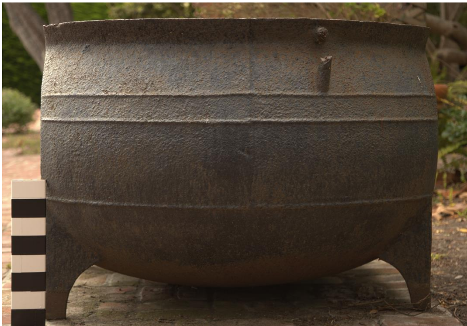
FIGURE 8: Metal block attached to repair damaged bottom leg of the northwest leg on Old Whaling Station trypot. Photograph by Jerome Riedl.
