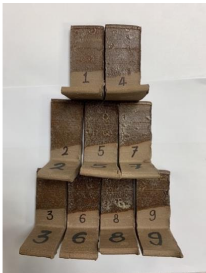
Figure 2: Tile test results of Greenville soil, soybean stalk ash, and felspar
