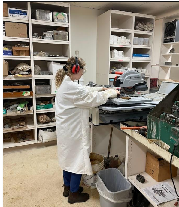
Figure 20. Cutting CR22 hand samples into 1/2-inch thick billets.
