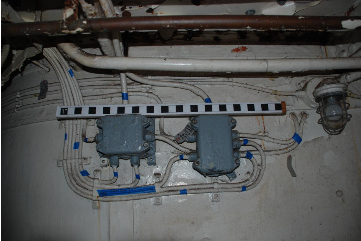
FIGURE 49. Scaled image shows two junction boxes and wires. The blue painter's tape was used to follow communications systems throughout LV83 . (Photo by author, 2010.)
