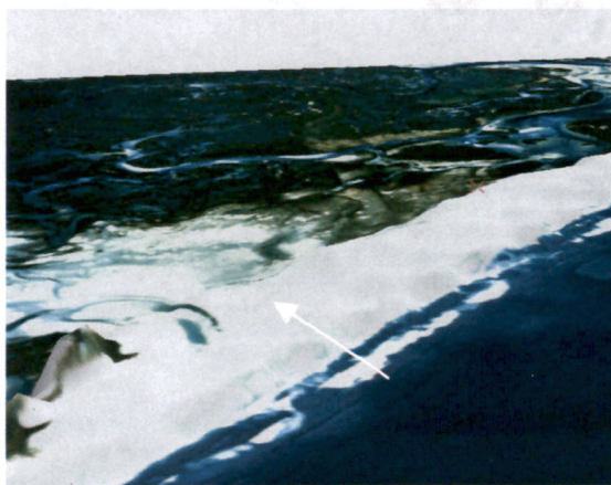
Figure 6. A digital visualization scene of the Old Topsail Inlet closure site (white arrow) produced by combining LIDAR derived DEMs (with a vertical exaggeration of 10) and USGS Color Infrared Digital Orthophoto Quarter Quads.
