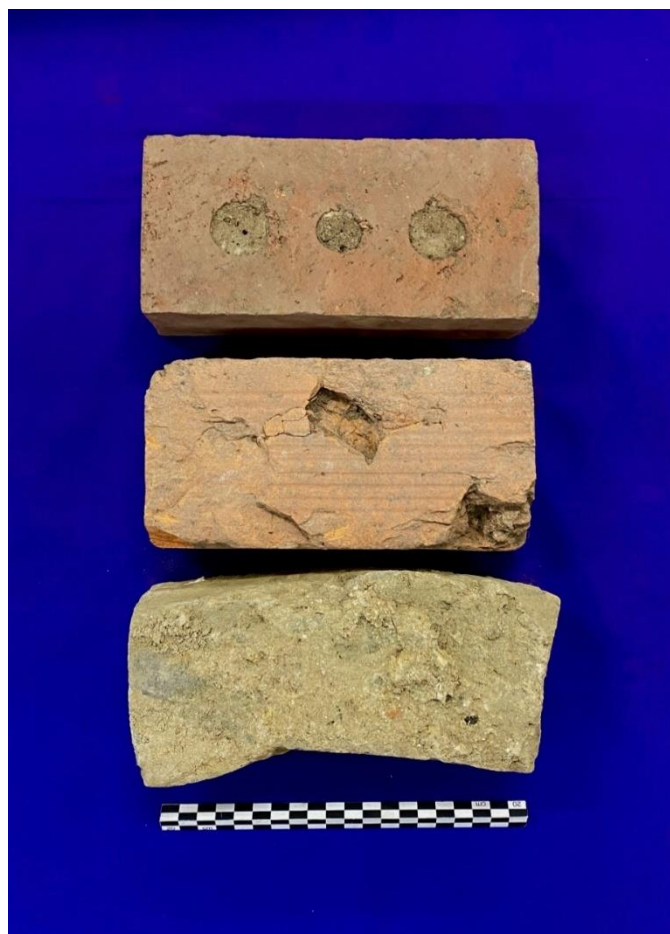
Figure 11: A side-by-side comparison of two machine-made modern bricks, above, and another handmade colonial type, below.
