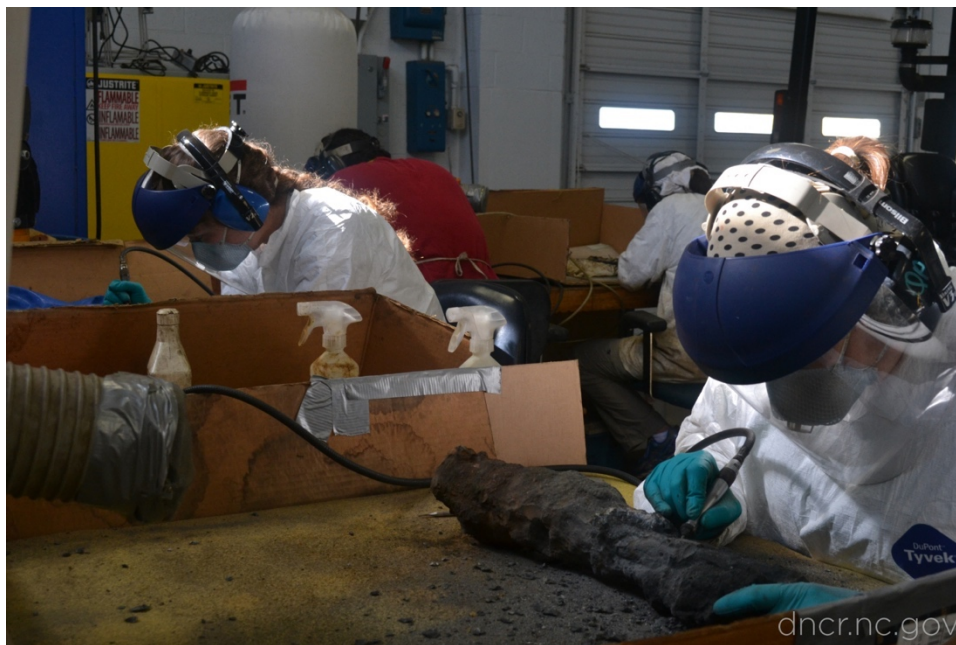
Figure 3. Conservators using airscribes to clean artifacts. Courtesy of NCDNCR.
