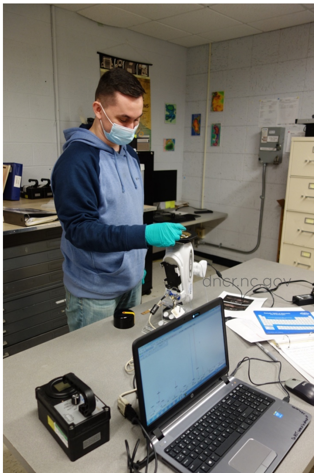
Figure 2. A Bruker XRF being used to x-ray an object. Courtesy of NCDNCR.
