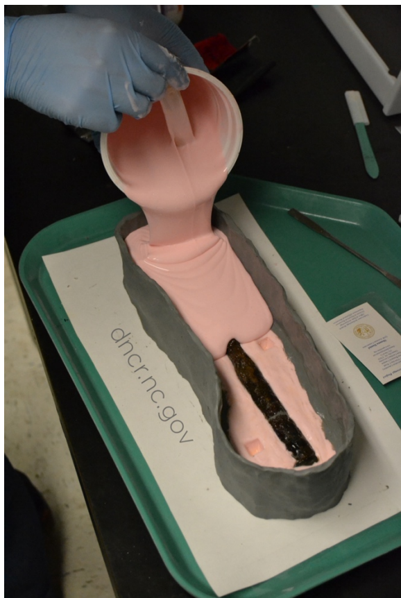
Figure 6. Silicone is poured over an object to create a mold. Courtesy of NCDNCR.
