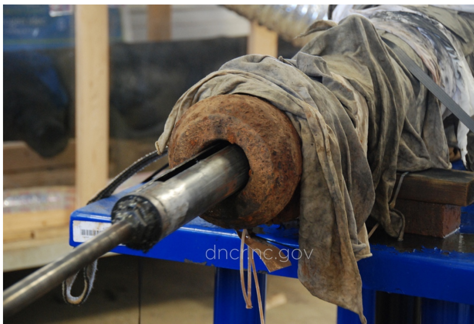
Figure 17. A metal tool is hammered down the bore of a cannon to unload it. Courtesy of NCDNCR.
