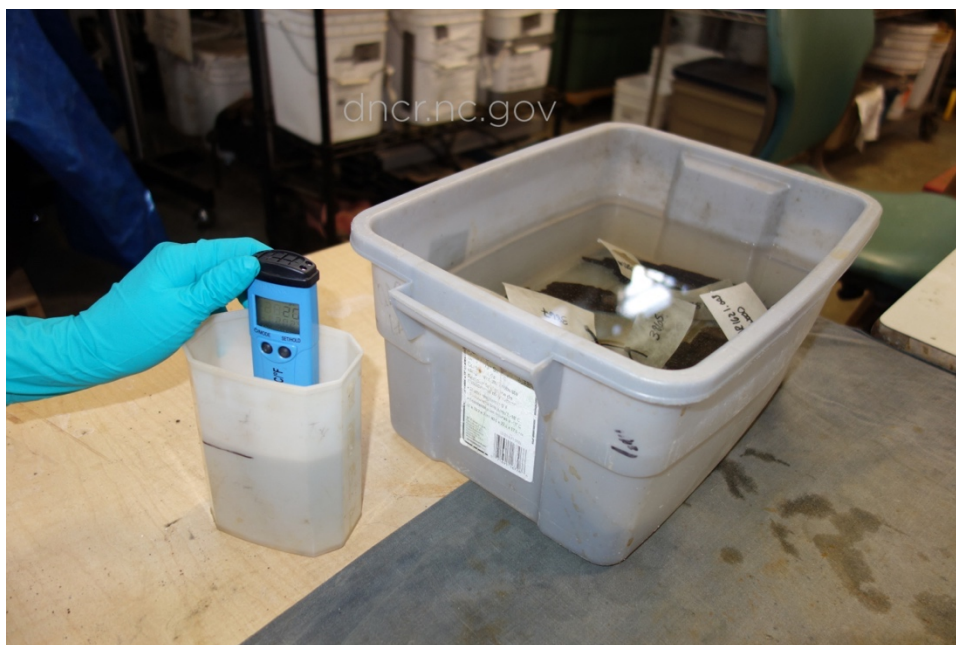
Figure 13. A TDS meter is used to test a solution. Courtesy of NCDNCR.
