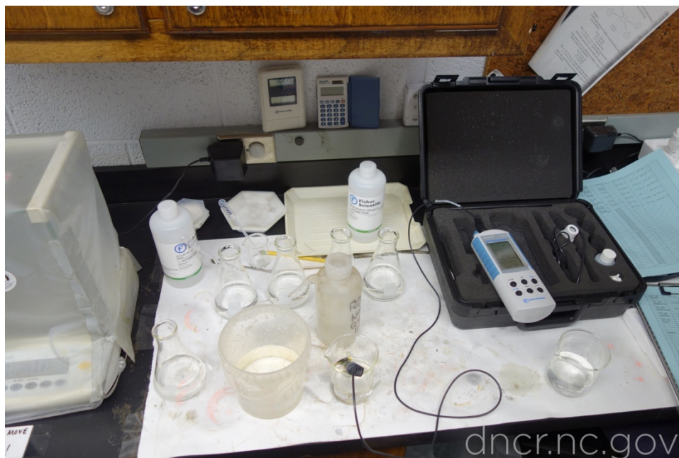
Figure 11. The Accumet meter and electrode measure the chloride levels of the sample. Courtesy of NCDNCR.
