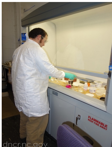
Figure 9. 100 mL of each tank sample are measured into beakers. Courtesy of NCDNCR.
