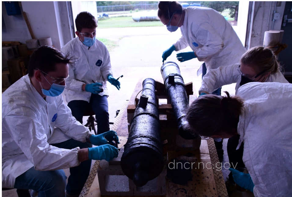
Figure 12. Tannic acid is applied to two cannons using toothbrushes. Courtesy of NCDNCR.
