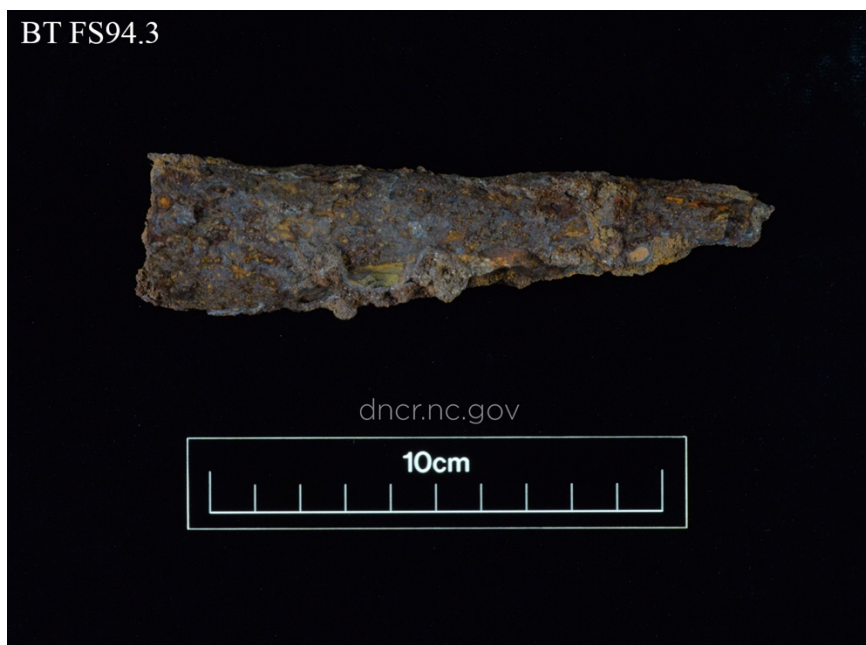
Figure 20. An iron fastener from Brunswick Town after being airscribed. Courtesy of NCDNCR.
