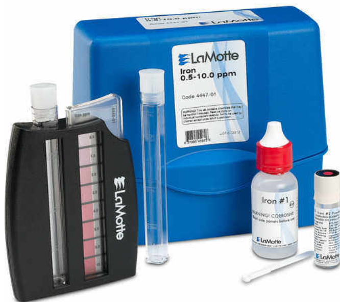
Figure 14. A La Motte Iron Testing Kit and all its contents. Courtesy of NCDNCR.
