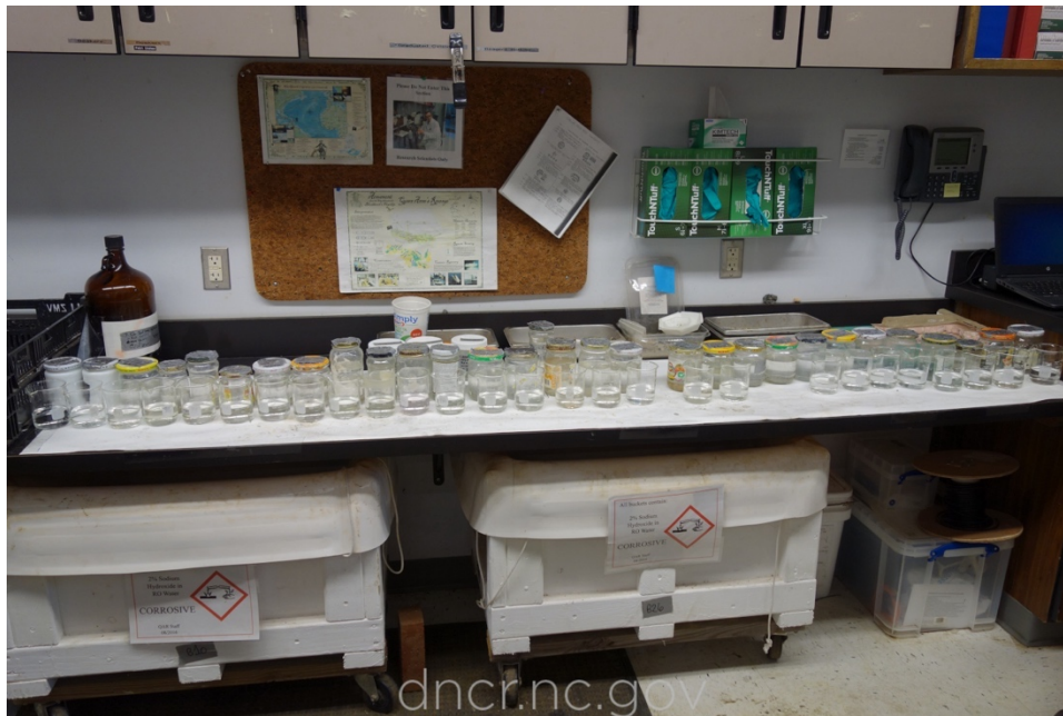
Figure 9. 100 mL of each tank sample are measured into beakers. Courtesy of NCDNCR.
