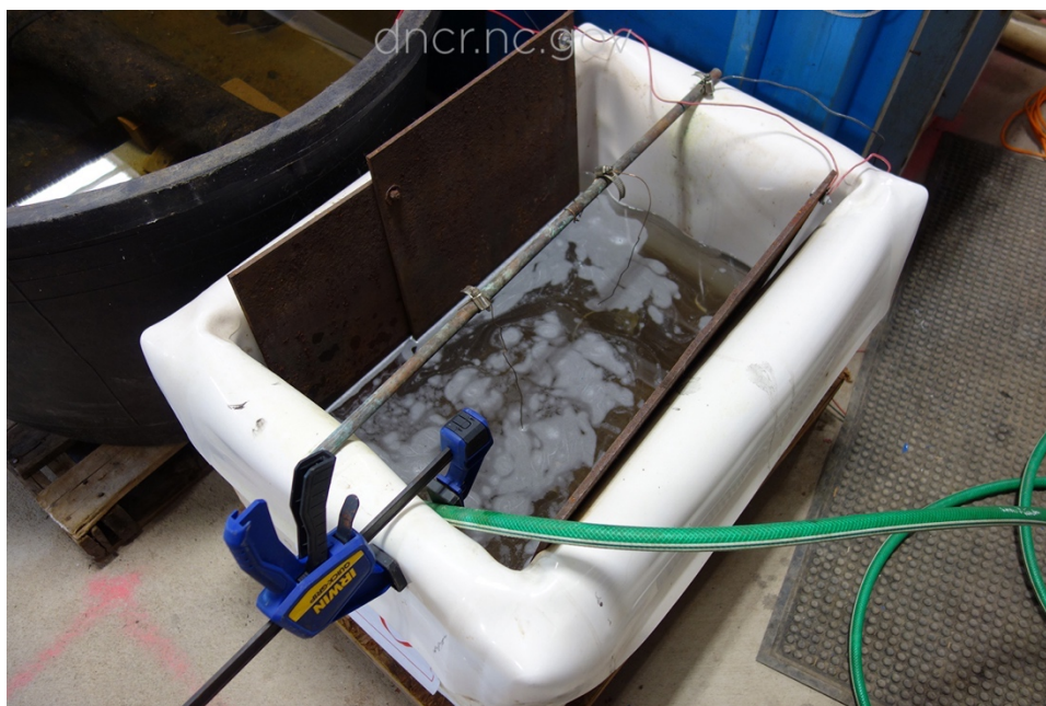
Figure 8. An iron artifact undergoes electrolytic reduction. Courtesy of NCDNCR.
