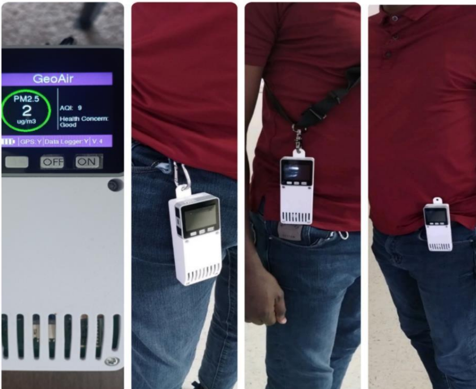
Figure 3.2 A GPS-enabled low-cost portable air monitor (GeoAir2.0) and the three ways to wear it
