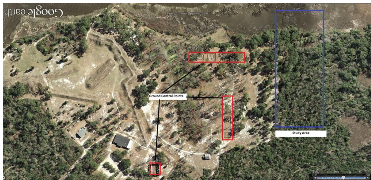
Figure 3.7 Control points for georeferenced map. St. Phillips Church (red rectangle in foreground)
