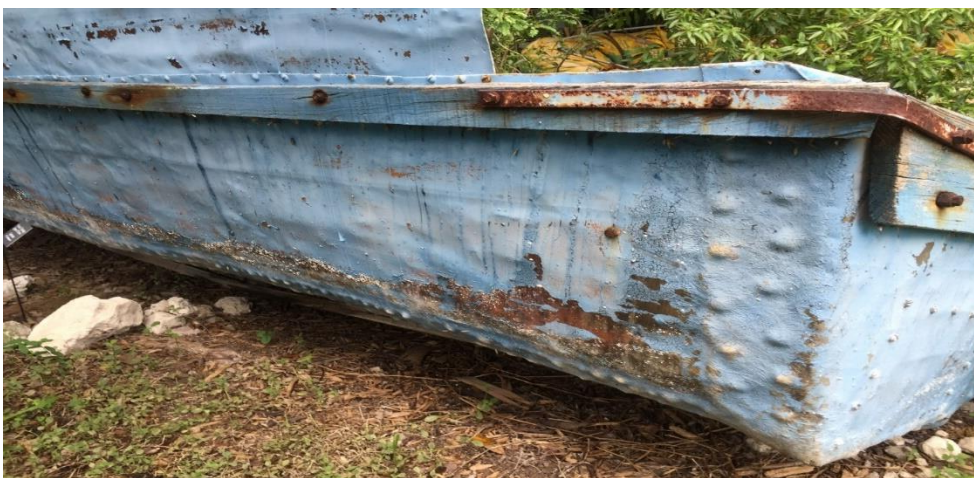
FIGURE 9 External of vessel with added freeboard; the bumps are bolts covered by fiberglass (photograph by author)
