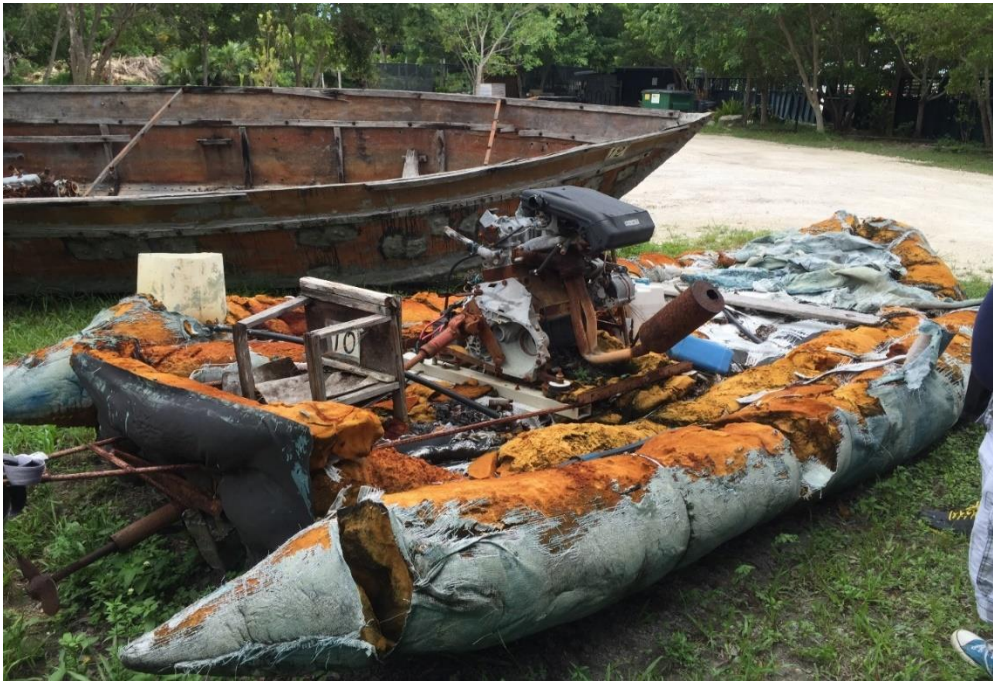
FIGURE 18 RHIB-styled vessel; note the handmade seat to operate a tiller (photograph by Richard McCusker)
