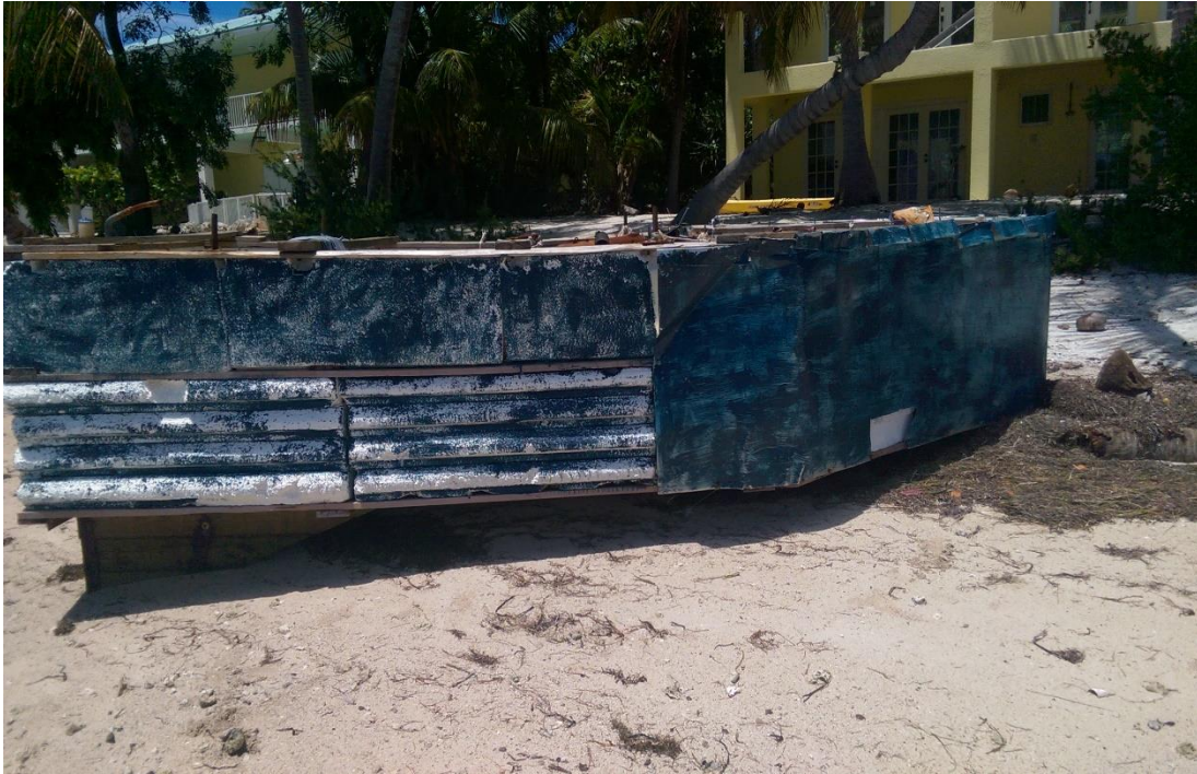
FIGURE 17 Foam vessel with aluminum on the bow (photograph by author)
