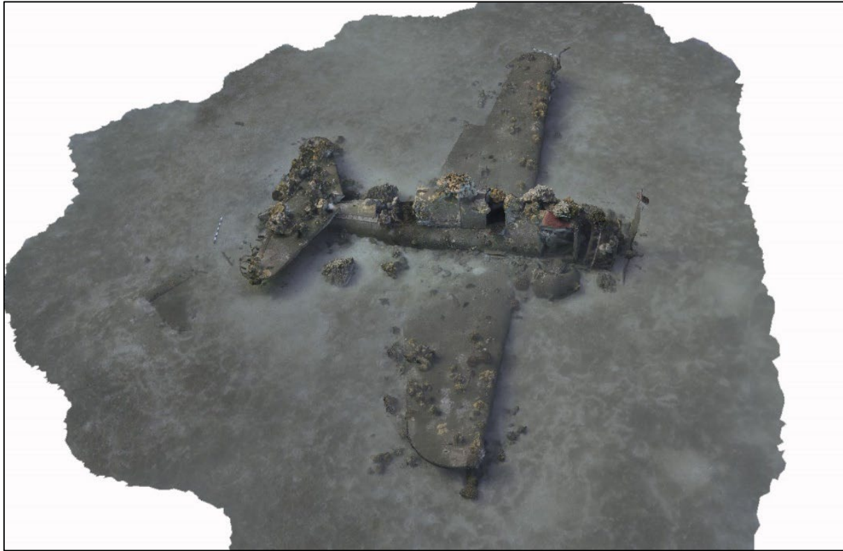
Figure 1.7. 3D photogrammetric model of SB2C-1C Helldiver site in Maui. One meter scale bar aft of the aircraft’s tail. (Model by the author, 2022)
