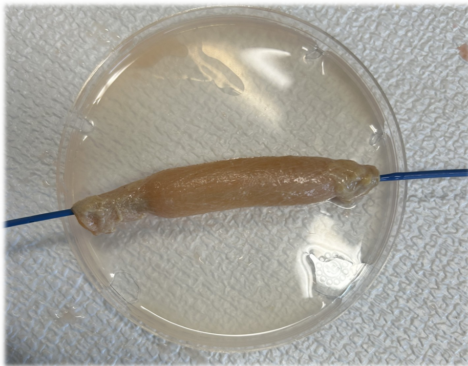
Figure 2 – Catheter being inflated inside of weakened vessel.
