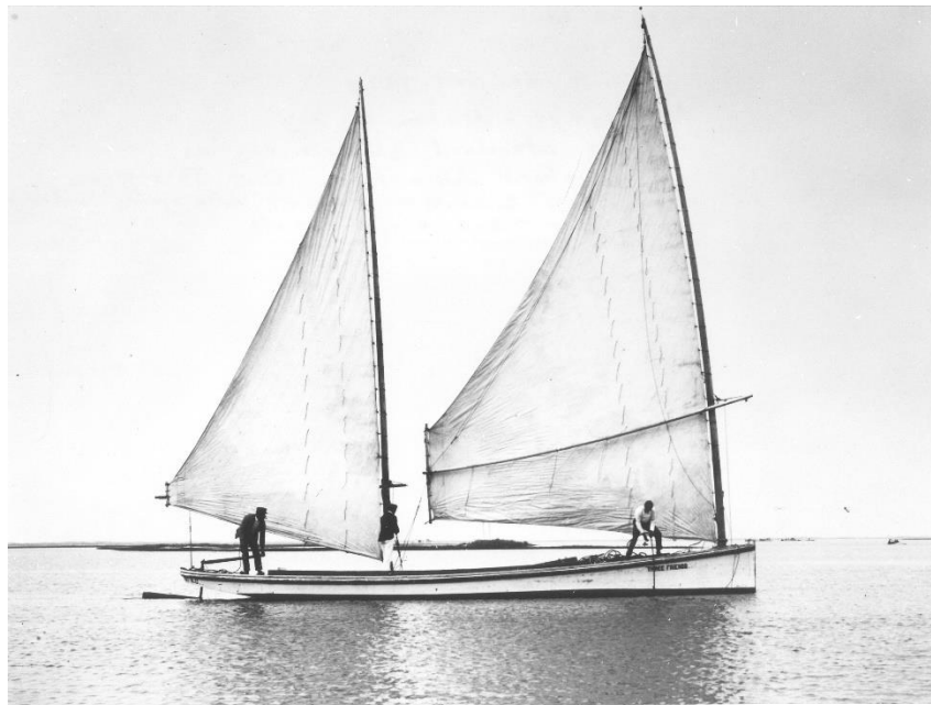
FIGURE 24. “Sharpie, The Three Friends ” built in Beaufort in 1893. 43 foot, Core Sound sharpie. Note the use of the two masted leg o mutton sails. (Image 78.086.039c) (Courtesy of the North Carolina Maritime Museum in Beaufort 2014).
