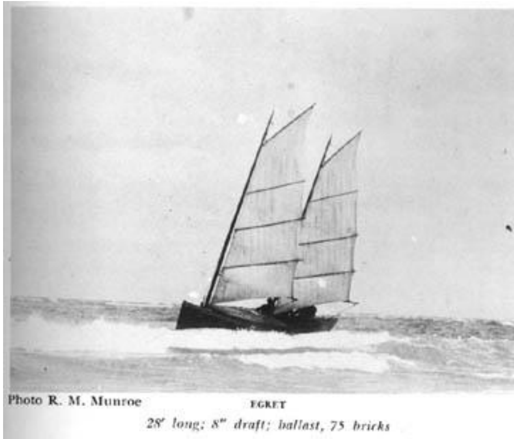
FIGURE 42. Photo of the Egret at sail. Note how close to shore she was sailing with no trouble, a testament to her extremely shallow draft and easy maneuvering with her unusual batton sails (Munroe 1886).
