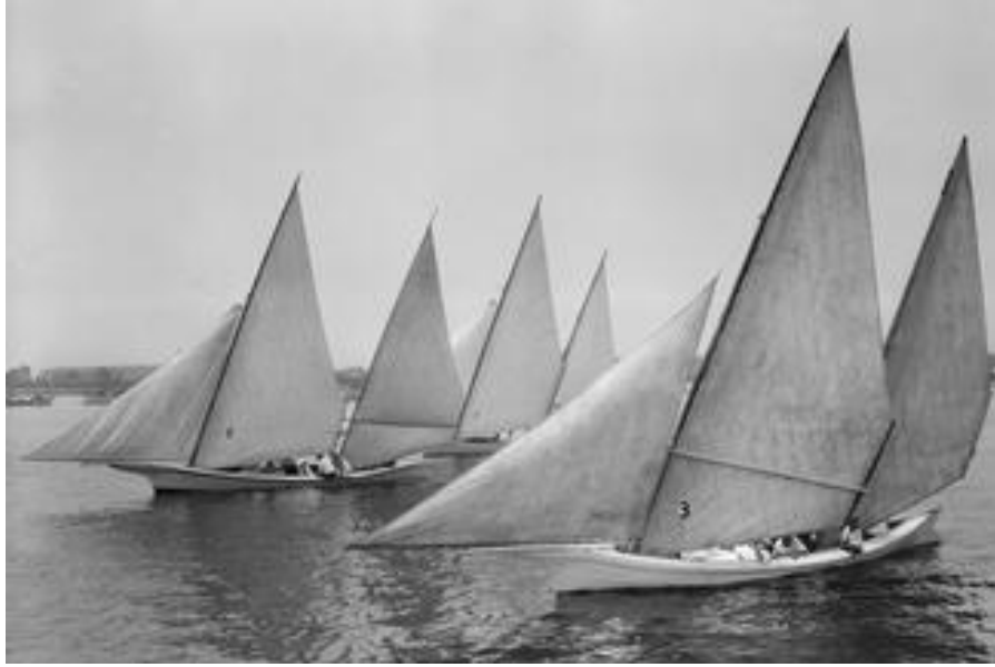
FIGURE 8. Typical Leg o' mutton sails at St. Michael's Regatta 1928 (Mystic Seaport 2014, Original image Rosenfield and Sons 1928) (Image 1984187.1984F)
