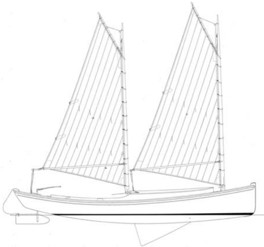
FIGURE 43. Drawing of the Egret. Note the definitive characteristics of the vessel: movable centerboard, narrow hull, shallow draft, and balanced rudder (Garant 2002).
