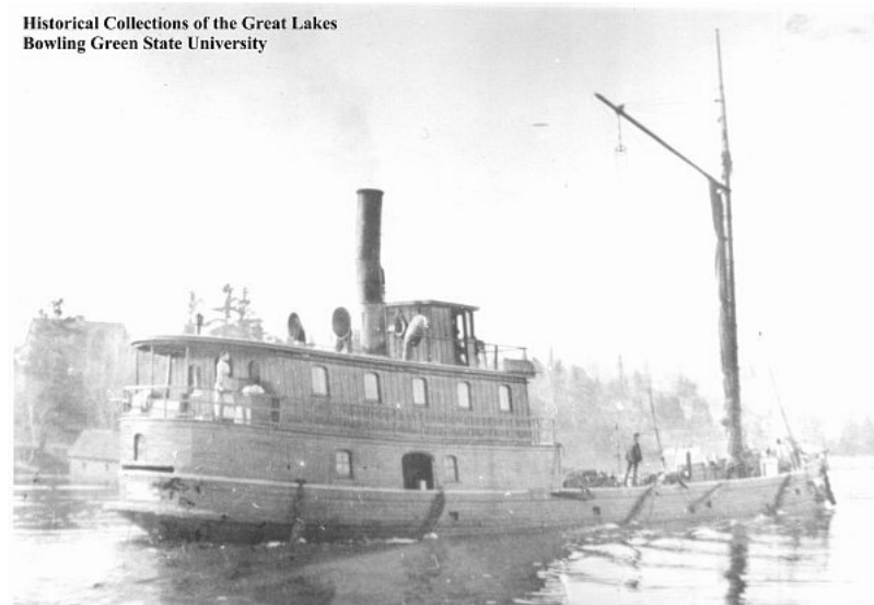
Figure 3-1: Aberdeen , a ship that was not selected, because of the visible open cargo hold and crane that marked it as a steam barge (BGSU).
