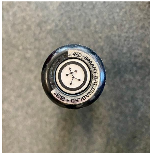
Figure 11: Blast Motion sensor bat integration. Blast sensor inserted into knob of Rawlings Quatro Pro BBCOR bat.
