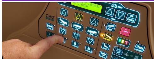
ACTIVATING THE BED ALARM | Step 1...
