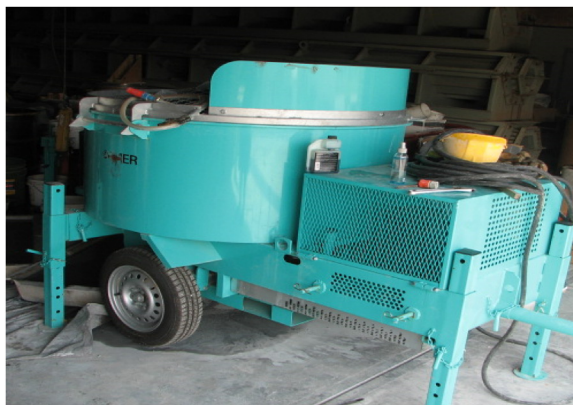
Fig. 1. High energy vertical shaft paddle mixer.
