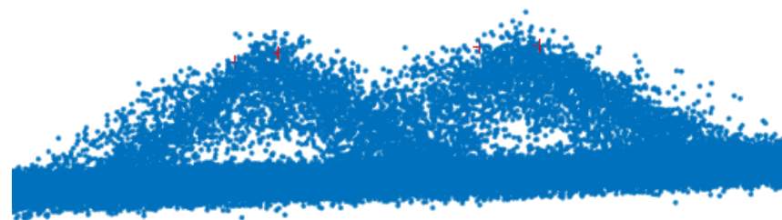
Figure 9. Zoomed-In View of Raw Point Cloud of Tent Targets with Four Survey Points Marked.
