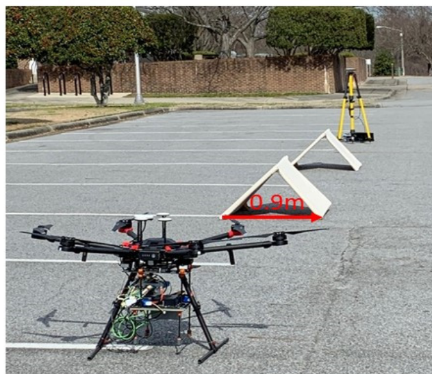
Figure 7. Experimental Setup for Model Validation with Tent Targets (Width = 0.90 m).
