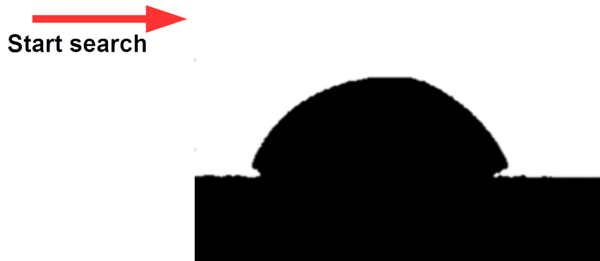
Figure 4.1: The mask was created to find the first black pixel in the image starting from the top, left as indicated by the search arrow.
